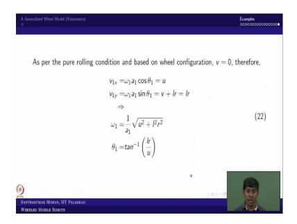
Now, further we will apply the pure rolling condition in the sense, you know like right these two wheels are actually like fixed wheel and although this is a fixed wheel with steerable, but these two are actually like fixed wheel. So, in the sense the vehicle cannot you can say slide on the lateral direction due to the infinite resistant theoretically applied on these two wheels.
