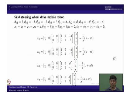
So, now, what we will try to do? We will try to find out  $d_1$  or in the sense  $d_{x1} d_{y1}$  to all the things. So, here what would be the  $d_{x1}$ ?  $d_{x1}$  would be small 1. So, d this is I am taking one two three four. So, in the sense  $d_{x1}$  is actually like this much which is 1 and  $d_{y1}$  is you call d.
