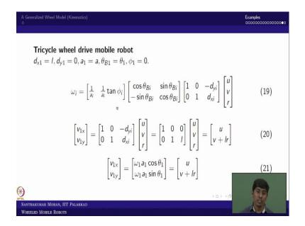
So, in the sense  $d_{x1}$  is  $d_{y1}$  is 0 and you know like the radius of the wheel is a and  $\theta$   $b_1$ ; here it is actually like rotated. So, in the sense you can see that the  $x_{ci}$  is actually like rotated with the angle of  $\theta_1$ ; in the sense, you can see  $\theta$   $b_1$  is  $\theta_1$  and there is no passive roller. So,  $\phi_1$  is 0.
