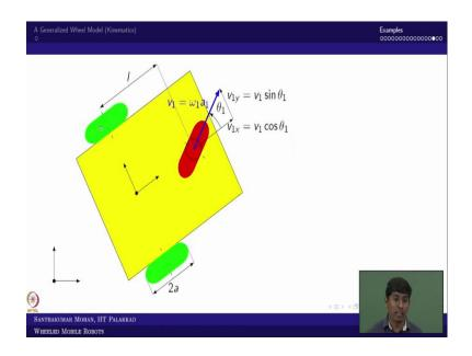
So, that is what address in this particular you can say example where you take one of the tricycle wheel model which is one of the olden auto style where the front wheel is drive and as well as steerable. So, in the sense you can see that  $\omega_2$  would be on the vertical axis, omega 1 would be rotated about this particular you can say axis.
