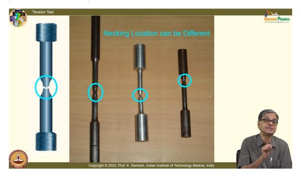
See, we have said it is an elastic continuum. That is an assumption or reality? It is an assumption. Reality is different, the material has some kind of defects, inherent defects. So, when you do the test, here I have shown it for a round specimen, in this specimen, it is more or less at the center. I have another specimen, it is not at the center, there is another specimen, the location is totally different. So, necking is precipitated by inherent defects, it can happen at any other point.
