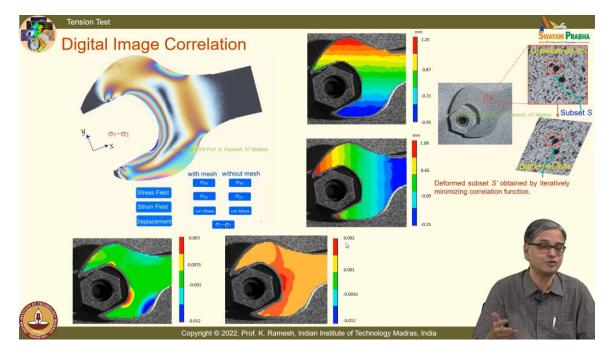
So, this summarizes. So, I have a speckled image. So, I take one photograph in the undeformed configuration. It is again an exaggerated picture. See, the spanner does not go through large deformation. So, the accuracy what you can anticipate in strain measurement is going to be poorer. It is not going to be as high as what you get under large deformation.
