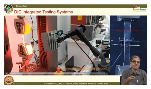
And if you look at modern instrumentation that comes with what is known as DIC integrated system, the expansion is Digital Image Correlation. So, you have a calibration of the measurement system here and then I would like you to notice the specimen is loaded and it is illuminated by a monochromatic light and you have two cameras that simultaneously record. So, you do not have a clip-on gauge or any such attached to the specimen and you directly get large value of strain.
