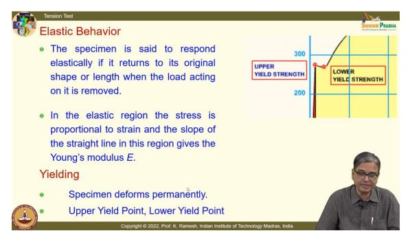
So, what is an elastic behavior? Suppose I apply the load and then release it. When I release it, it will come back in the same loaded path and it will come back to its original position. What was happening in the case of a rubber? When I had taken the rubber band and I stretched it, I could go up to 250% very very comfortably and release my hand, it was coming back.
