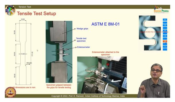
And you know, you have standards available. You have ASTM standards. And they give you what should be the dimensions for a flat specimen like this. And you have a sufficient length for you to grip the specimen. And you also ensure that you provide a generous fillet so that this is a test section and the test section fails in an experiment.
