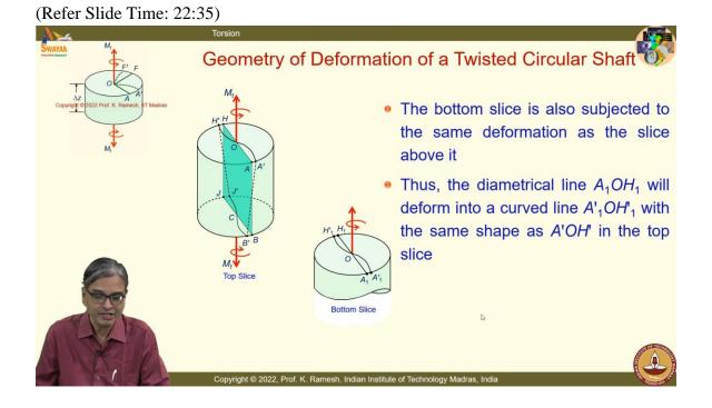
See the bottom slice is also subject to the same deformation as the slice above it which we have already noted and it should also be like this. So, the diametrical line  $A_1 O_1 H_1$  will deform into this. But these two are different.
