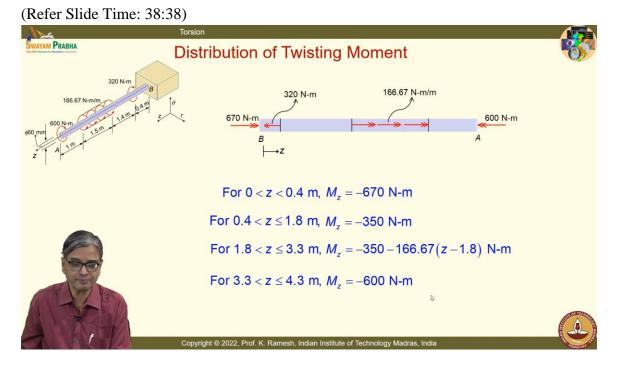
So, that is shown in the right direction in the diagram. So, for the zone 0 to 0.4, see we are analyzing from end B. So, we are analyzing this section. So, you should understand how the drawing is drawn for convenience. So, in this section, you take a cross section and then write the free body diagram.
