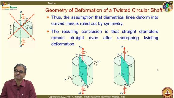
The only way that it can deform is a line OA will deform to another straight-line OA'. Is the idea clear? This is by thought experiment.
