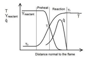
This zone is called the preheat zone. Reaction zone exists next to it. Reaction zone has a very small thickness; order of a milli-meter. Towards the end of the reaction zone, a bright or luminous zone is present. Here, the temperature is maximum (flame temperature,  $T_f$ ).
