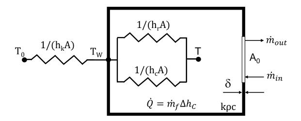
In case where  $T_w \approx T$ , the heat flux is expressed (by solving transient heat conduction) as,
