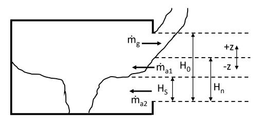
Smoke layer has descended to a particular height from the ceiling,  $H_s$ . measured from the bottom of the vent. Below this, air from atmosphere enters. Above this level, a neutral plane is formed at a height of  $H_n$ , measured from bottom of the vent. Above  $H_n$ , hot gas leaves and below  $H_n$ , air comes in.
