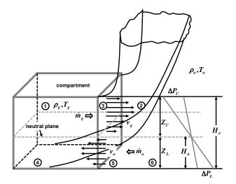
Flow of gases in & out of an enclosure during fully developed stage
