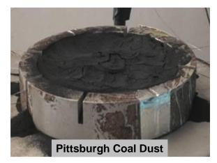
Coal dust after the test where ignition criterion is positive – experiments conducted in WPI, MA, USA.
