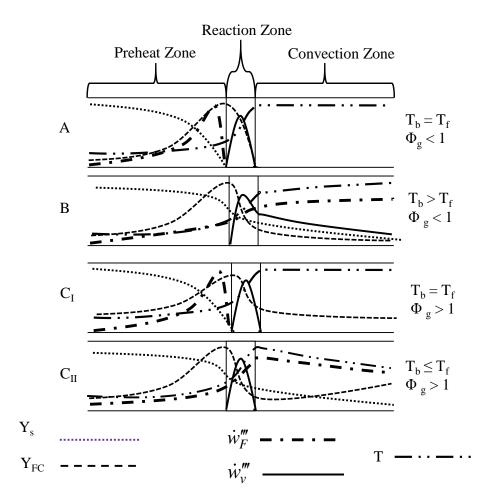
$Y_{S} = mass fraction of solid$   $Y_{FC} = mass fraction of vaporized fuel$   $\dot{W}_{F}^{\prime\prime\prime} = reaction rate$   $\dot{W}_{\nu}^{\prime\prime\prime\prime} = vaporization rate$   $T_{b} = convection zone temp.$   $T_{f} = reaction zone temp.$
