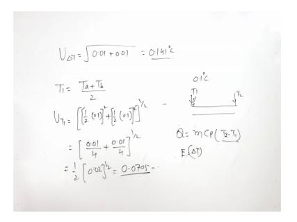
So, when we take 0.1 square, then it becomes the uncertainty in delta T uncertainty in delta T is equal to under root of 0.0 1 plus 0.01. Now, if we take under root of 0.02, it becomes 0.141 degree centigrade right. So, temperature difference individual measurement is 0.1 and 0.1 right. So, it is not 0.2, it is 0.14141 degree centigrade in uncertainty measurement of delta T.
