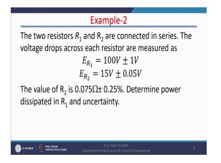
Another example is, if 2 resistors R 1 and R 2, they are connected in series. So, I will rub this one. There 2 resistors R 1 and R 2, they are connected in series. This is R 1 and this is R 2 right.
