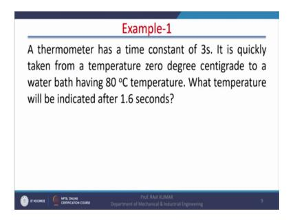
Now, we can take one example. Now, in this example, it is stated that a thermometer has time constant of 3 seconds. So, time constant for thermometer is three seconds right.
