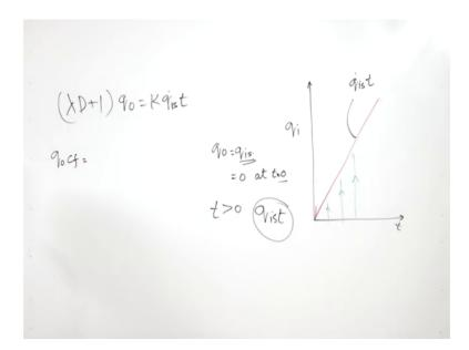
Now, the basic equation is q o is equal to q i 1 minus e raised to the power minus t by lambda. This is the basic equation for first order system. Yes, here we have to multiply by sensitivity also q o is equal to K q i fine. Now, q o is equal to q i s is equal to 0 at t is equal to 0 initially both are 0 right and input to the instrument into input to the instrument is rate multiplied by t suppose rate of input is q i s dot. So, instantaneous input to the instrument is q i s t.
