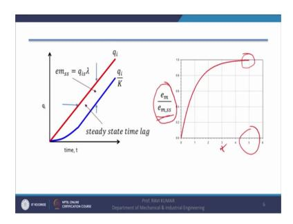
Now, regarding this error in measurement in this graph the same thing is shown here in this graph. This is error in measurement divided error in measurement at steady state and this is increasing and it is the ratio is attaining at the value of one at approximately t by lambda is 0.5 is now it is not t by lambda it is it is t only. So, at after 5 seconds right.
