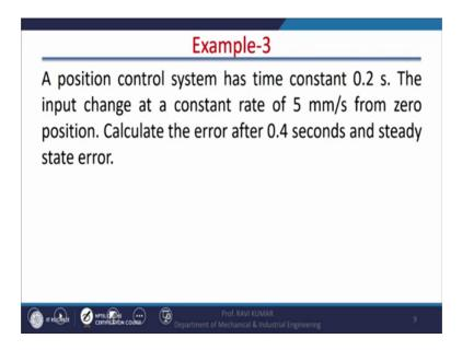
The statement of the example is a position control system has time constant 0.2 seconds. So, time constant lambda is 0.2 seconds. It is for position control system. (Refer Slide Time: 27:22)
