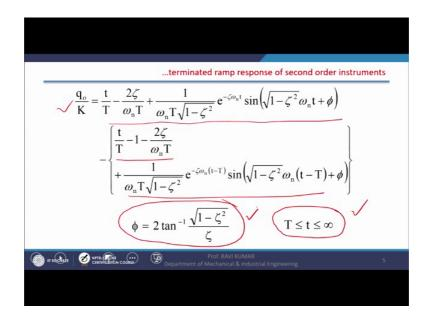
So, now here after just putting these boundary conditions here as shown here we get the output q by K is equal to t by T, then 2 zeta by omega n plus 1 by omega nT under root one minus zeta square e raise to power zeta omega nT then signed under root one minus
