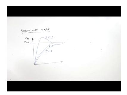
So, error in the measurement for second order system ramp input is going to be zeta is equal to 1.5, it is going to be like this for zeta is equal to 1.5, this is over damped system for a critical damped system.
