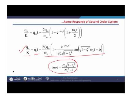
So, normally our systems second order systems are followed by the equation governing equation by under damped system and that is qo by K this is rate of input minus this expression the angle phase angle can be calculated by using this equation which is a function of damping ratio.
