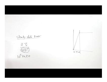
Now, steady state error sse, the steady state error is of the size of two zeta divided by omega nT. So, in terminated ramp response there is an a steady state error and steady state error can be expressed by this, Now here if the T is very small, if we make omega and very high even for that if T is small and the product has to be high higher than much higher than the zeta, then steady state error will be reduced.
