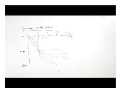
Now, phase angle is always negative as I say that the response cannot lead the input. So, it is always negative to 0 and it will go up to minus 180 degree, but in phase angle also 90 minus 90 is important, I will draw a one line at minus ninety degree and 1 line will draw at 1 here and then it can be 1, 2 and 3, 4 and so on right.
