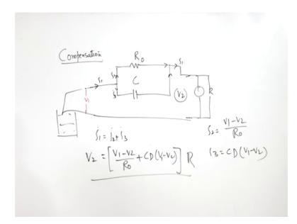
So, I 1 is equal to I 2 plus I 3 and this is going to be equal to V 1 minus V 2 upon R o plus C D V 1 minus V 2. And this V 1 is equal to this current multiplied by R, V is equal to IR this is not this is not V 1, V 2; V 2.
