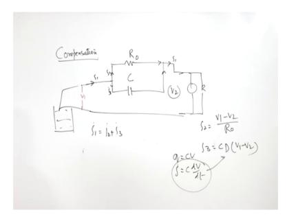
So, here, again I will write I 1, I 2 is going to be equal to V 1 minus V 2 upon R o and I 3 is going to be equal to C D V 1 minus V 2 because resistance of display unit also has to be taken into account right.
