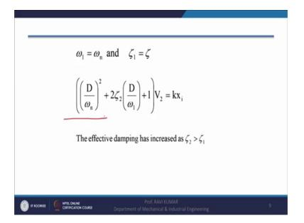
And here we can see that the effective damping, the zeta 1 is equal to zeta, omega 1 is equal to omega n and this equation can further be modified as this one and here the effective damping has increased from zeta 2 to zeta 1 to zeta 2 right.
