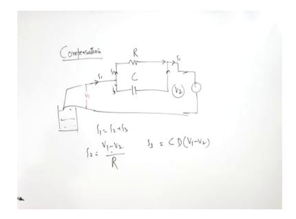
There is a suppose some fluid and the temperature is the fluid is being measured with the help of a thermocouple, thermocouple is giving output let us say output is, so output of this thermocouple is let us say V 1 right.
