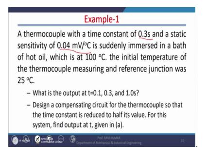
Then it is being asked, design the composition circuit for thermocouples. So, that a time constraint is reduced to half it is value right.
