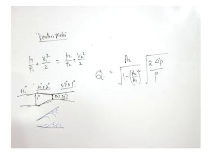
Suppose this diameter is 1 inch. So, upstream side has to be around 10 inch length without any change in the diameter right. So, it has to be a stabilized and the stabilized and the fully developed flow and, the converge angle in order to reduce the loss is the converge angle has to be 21 degree plus minus you can take, 1 degree or 2 degree 21 degree plus minus 2 degree has to be angle of convergence. Diverging angle has to be 5 to 7 degree plus minus 1 degree.
