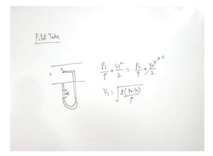
When you want to have flow rate in a pipe suppose, I want to measure flow rate inside a pipe I will use this method from here, I will make a tap for static pressure here, I will make a tap for dynamic pressure, right it they will be connected through a u tube
