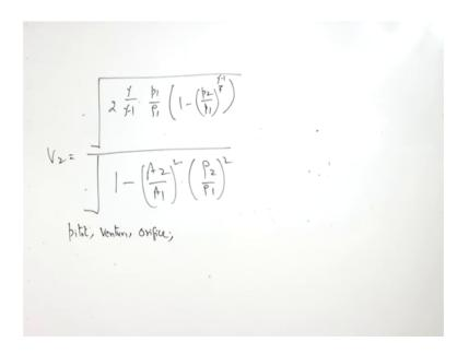
Now, using this equation the final expression can be written as V 2 is equal to under root 2 gamma over gamma minus 1, multiplied by p 1 minus rho 1 1 minus p 2 by p 1 is to power gamma minus 1 whole gamma divided by under root 1 minus A 2 by A 1 whole square, multiplied by rho 2 by rho 1 whole square right.
