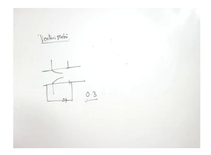
Now, in orifice meter there is no converging or diverging passage, there is a plate which has a circular orifice in the middle right and, working principle is same pressure static pressure here, because here there is there is going to be fall in the static pressure, but in this case and then we take the delta p, I think these instrument you must have studied in the classes of fluid mechanics also that is why am discussing in brief, am not going into the details in orifice meter.
