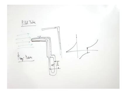
Here there is going to be a nose for a stat stagnation pressure and, it is covered by another tube. So, not a tube another layer of metal and, it has holes like this it is a hole and, then it is coming this way this side. Now, here this is filled with the static air, suppose this air is the medium this is filled with static air.
