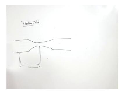
Right it also works on the principle Bernoulli's theorem or, it also works on Bernoulli theorem. In venturi meter the flow meter the physically the flow meter appears to be like this right, there is a upstream pipe and there is a downstream pipe also of constant cross section right.
