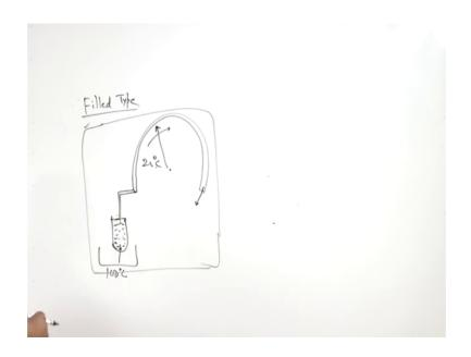
It is filled with some fluid may be a liquid or gas and it is connected to broaden tube as I explain you earlier it is a curve tube right when this broaden tube is connected with this right when this in this bulb it is closed. So, when in this bulb there is a energy addition by virtue of temperature difference or it comes with the contact with the measure end the liquid expands or the fluid expands and this fluid causes the extension of free end of the broaden tube in this direction.
