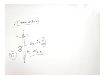
So, what we can do? We can take one slab I mean we can take one slab and in this slab, we will, I will just give you we can take one slab, right and heat this side is heated and heat transmission takes place. Q thickness of the slab is known, X temperature on the both sides we can measure by T 1 and T 2 and this is the constant heat flux, right.
