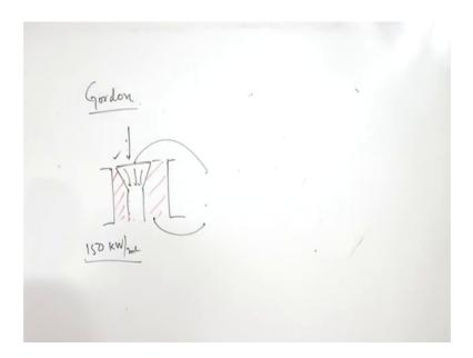
The heat flux meter is embedded in the wall. It is a constant end surface, right. A copper wire is fixed here and this is all copper. This is all copper, right and one copper wire, the copper wire is fixed here, right and when the heat comes in this direction, the transmission of the heat in the radial direction is measured, right.
