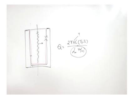
Two, cylinder method is used, there are two cylinders. Cylinder 1, this is one cylinder right and inside that there is another cylinder, right. From the top they are insulated. They are insulated at the top. So, insulation is here. Both the cylinders are insulated, right and there is a gap between the inner wall of the outer cylinder and outer wall of inner cylinder. Now, this gap is very small.
