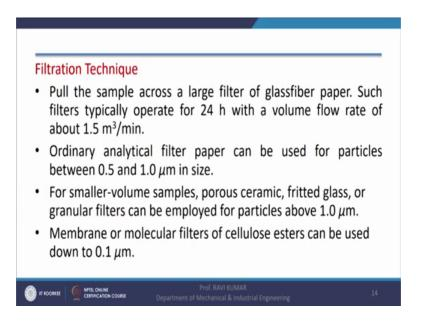
A glass fiber paper can be taken a glass fiber taker paper can be taken and this glass fiber type of paper the sample is pass through this paper for 24 hours right.
