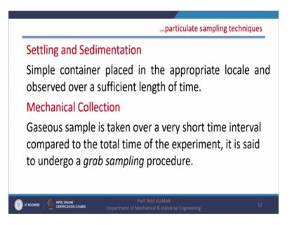
Now settling and sedimentation and there is the 2 techniques, settling and sedimentation and mechanical collection. Separation of the particles first is settling; settling in sedimentation if I said earlier if the particle size is large it will settle and it will and it can be collected at one type if the sufficient length of time is given for the settlement. So, the sample is taken and it is left for a long time left for a long time, let us say 24 hours or 48 hours.
