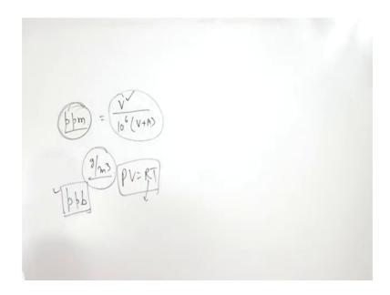
So, it is volume to volume ratio parts per million is volume to volume ratio. Another way of expressing the pollutants is, grams per meter cube that is expression in the basis of unit, which is based on the mass grams per meter cube or it can be expressed in terms of ppm.
