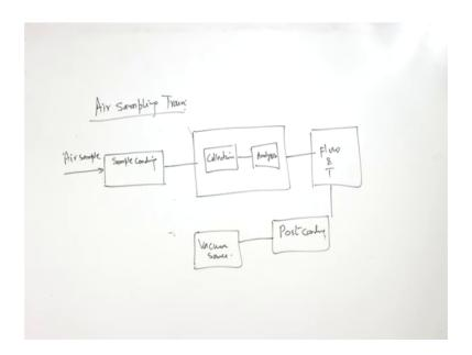
So, in air sampling train the there is one inlet for air sample. Now this air sample will go to the sample conditioning unit sample conditioning right. Now after sampling conditioning it will go to the sample collection unit, and sample connection unit is normally having 2 parts first of all collection and second is analysis; analysis also done here and this is this is a part of sample collection right.
