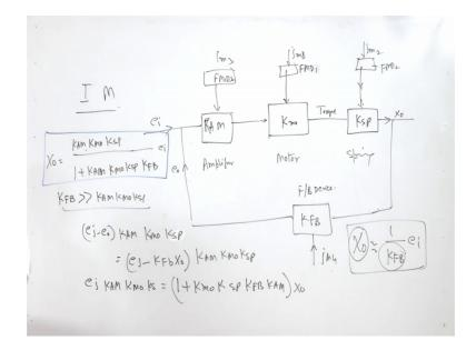
So amplifier right. So, amplifier will also have F or K and this is EI or this amplifier will also have some spurious input. So, this is also IM3 right. Amplifier this input signal will go to the amplifier then it will go to the motor then it will go to the spring. And part of this signal will be taken back and this is a feedback this is amplifier. This is motor and this is a spring.
