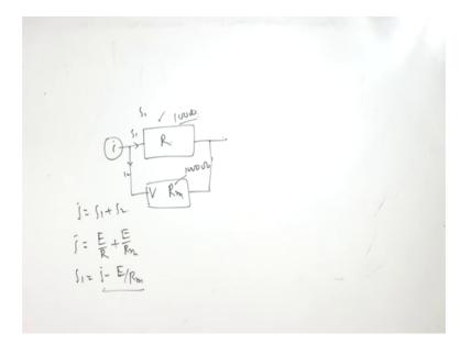
So, i is equal to let us say that, the current is splitted in 2 parts i is equal to i 1 plus i 2 this is total current it is i 1 and this is I 2 and potential difference between these 2 is E. So, i is equal to E by R plus E by R n because they are connected in parallel. So, E is will remain common or we can say that current here i 1 or E by R i 1 is equal to i minus E by R m right because R we do not know r we do not know, but we have measured the I 1 right.
