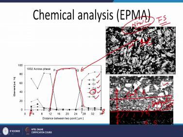
This is an just an example of the line scan analysis like say this is the Nickel tungsten carbide coating deposited by the flame spraying method and the scooting is having primary tungsten carbide and other dark one is the eutectic matrix. So, here the analysis is performed between
