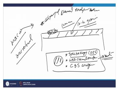
There are two broad aspects related to the chemical analysis one is like macro level analysis and another is macro level analysis. So, in case when a surface which has been modified like this so for macro level analysis we select one big area like say maybe of the 10 mm in diameter which will be having the 10's of the 1000's of the grains are the micro constituents. So, average composition of that particular zone is achieved and it indicates the average composition of the modified zone.
