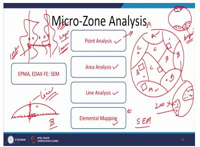
And these techniques are these are the four techniques which are used for micro zone analysis 1 is called point analysis and another is area analysis 3rd is line analysis and 4th is element analysis and each one now we can I will try to understand like say this is the area which is under focus at a magnification of say 200 X. So, we are able to see various micro constituents under the scanning electron microscope.
