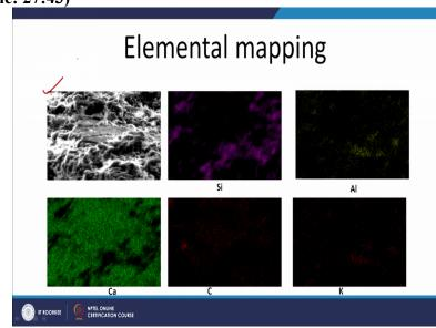
Similarly this is the elemental mapping for another and kind of the fracture surface which is showing where the silicon is present where Aluminium is present where carbon is present sodium or potassium is present and calcium is present. So, elemental mapping helps us to see for a given microstructure it helps to see where which element is present. So, elemental mapping helps us to see for a given microstructure it helps to see where which element is present. **(Refer Slide Time: 28:05)**
