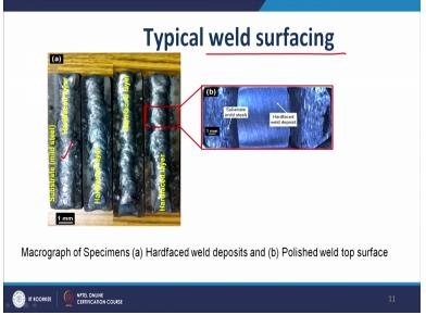
As far as the characterization metallurgical characterization is concerned will take up the example of the weld surfacing, so here the weld hard facing is on the mild steel substrate is carried out and we take to the sample from this zone and it analysis was performed. So, here both sides we have the substrate of the mild steel and in between there is weld surfacing deposit. **(Refer Slide Time: 31:12)**
