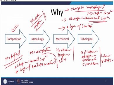
So, these slide shows that for a given modified surface of a particular composition will have a set of the metallurgical properties with regard to the microstructure especially and this microstructure will be governing the mechanical properties such as hardness, toughness, work
