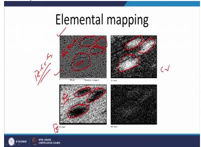
I was talking about the elemental mapping like say this is the microstructure of the hard facing coating where the matrix is of the eutectic and it is having the carbide particles like chromium carbide particles. Wherever chromium carbide particles are present like this elemental mapping is carried out for chromium will see the bright particles in the zone where is present. And other locations and when the analysis done for the other is this was the iron chromium carbide weld surfacing.
