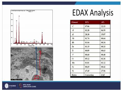
Similarly this is an indicator of the aerial analysis, for aerial this is this is the area which was selected in it was analysed this is showing that diffraction pattern achieved through the EDX analysis.
