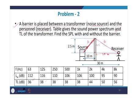
So, the problem 2 here is that, we are given a barrier is placed between a transformer which is noise source here and a personnel who is the receiver and the table gives you the sound power spectrum. So, here the L w is a function of the frequency and it is given a set of values; and the transmission loss is also function of frequency, it is given as a set of values.
