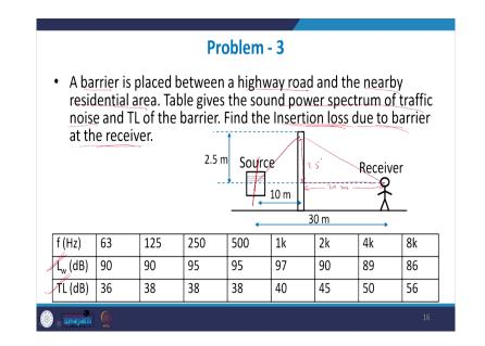
Last problem for this session, this is going to be a problem on highway barrier. So, we are going to find out, this is a question on the insertion loss of a highway barrier.
