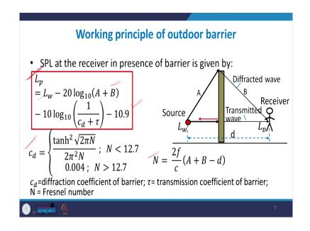
And when the barrier is present between the source and receiver in that case the SPL at the receiver is given by L w, which is the power level of this source minus 20 log A plus B; here this is the distance of A plus B, which is measured from source to the barrier edge and then from value edge to the receiver minus 10 log of 1 upon c d plus tau minus 10.9.
