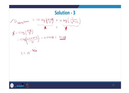
So, for the highway barrier, I L for a highway barrier comes out to be 15 log A plus B by d plus 10 log of 1 upon c d to the power 3 by 4 plus tau. So, this is the expression for the highway, insertion loss due to highway barrier. So, let us first calculate this value.
