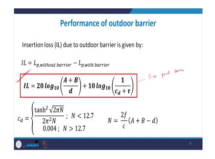
So, now, we have this L p without the barrier and L p with the barrier. So, the insertion loss you when you subtract the two expression, it comes out to be this ; this is for a point source assumption. So, the source is small.
