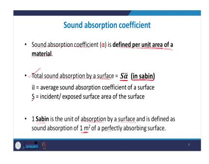
So, alpha comes out to be per unit area of the material. So, we have whenever we have a sample and we are measuring the sound absorption coefficient value for a particular material sample. So, by definition this alpha gives us the value of what is the absorption per meter
