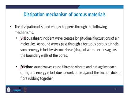
The second form of dissipation is in the form of fiction. So, as the sound waves enter and let us say the fibres they are loosely bonded together they are not solid like a solid table or anything. So, when the sound wave is passing through as a longitudinal oscillation that the fibres through which it is passing by they will come into contact with it and they will also start to vibrate.
