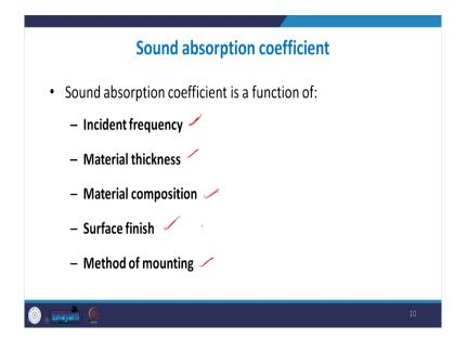
So, the alpha value now depends on many factors. It depends upon what is the incident frequency. It also depends on the material thickness. So, when we were discussing about the alpha value for the particular material then nothing was mentioned about what is the surface area of the material or the thickness. So, now we know that when alpha value is mentioned that means, that it is considered for a unit surface area of a material, but what about the thickness.
