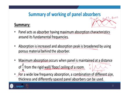
So, to summarize the panel absorbance they act as absorber having a maximum absorption characteristic at its fundamental frequencies and this absorption can be increased and the peak can be broadened if you use some porous material behind the absorber. And the maximum absorption is obtained when the panel is maintained at a distance of lambda by 4 from a rigid wall or a floor or a ceiling whatever and because this panel it has some fixed resonant frequencies.
