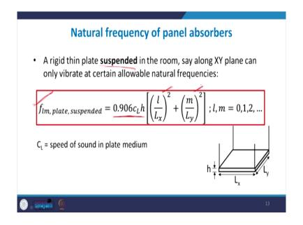
Then the natural frequency of a suspended panel can be given by this equation this is the equation which we get if we solve it. Anyways the cell the derivation of this is not within the scope of this course. So, only the working of these materials and their advantages and limitations are. So, I am directly giving you the expressions.
