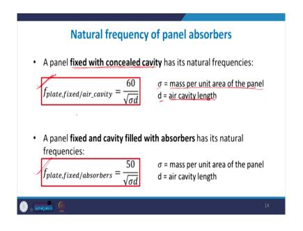
So, I am going to straight come to the approximate solution. So, suppose we have a fixed panel with a concealed cavity which I had showed you. So, the natural frequencies of this panel comes out to be 60 by under root of sigma d. So, this is the approximate this is after calculation an approximate solution is derived. Here sigma is the mass per unit area of the material and d is the air cavity length. So, if we go back to the figure.
