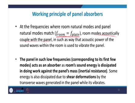
So, how does this panel absorber work. So, whenever we have placed the panel inside some room or any closed area and some sound is generated within that room. Then now we know that the room itself has it is natural frequencies and therefore, these sound waves will be the sound the SPL will be the highest at these natural frequencies because that is where the resonance will take place and a heavy amount of vibration the particles will oscillate with almost infinite amplitude.
