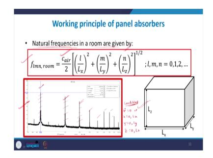
So, when we have a room. So, in a room inside a room the natural frequencies of a room are given by this expression and this can be very easily derived just the way we derived the expression for the sound waves inside a long tube. So, what we assumed there was that both ends are rigid and at the rigid end the particle velocity becomes 0.
