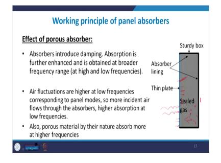
So, that is what happens. Now, if we fill this panel with the absorber material then what we are doing here is that sound wave is being incident on the panel. The panel starts to vibrate to and
