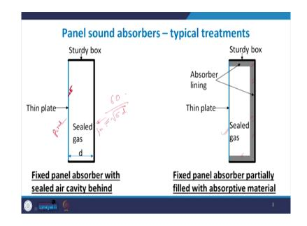
So, these can be used in various different ways. So, now, you already know the schematic for a suspended absorb the suspended panel. So, you have a panel which is hanging from some structure either along the 4 corners or also just from one side as we saw in the last case. And for a fixed panel how does it look like let us see what does a fixed panel look like from inside. So, a fixed panel from inside looks like this.
