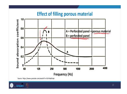
So, in that case this will be a typical curve. So, this is a sharp peak when there is no just a perforated panel and when you add a porous material to it, you get a more broader peak. So, although the intensity absorption intensity is reducing, but the peak is broadening so that is the effect of adding a porous material.
