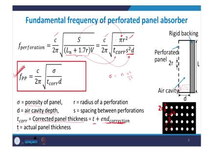
So, with this what we see is that this is the expression for a Helmholtz resonator when we make an and the locus comparison c by 2 pi and the net surface area enclosed. So, the net
