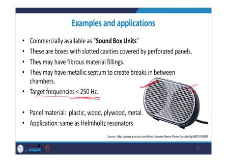
And what are some of the areas where such resonators can be used? Now you have if you have seen you will see that commercially there are lot of sound box units and this figure shows a typical example of a sound box unit.
