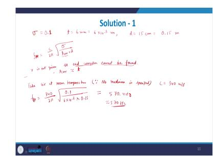
So, all these values are given to us. Let us write down these values sigma is given to us or the open area ratio is 10 percent. So, infraction it will be 0.1, thickness is given of the panel is 6 millimeters which is 6 into 10 to the power minus 3 meters.
