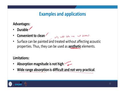
So, a few example advantages and limitations are first of all they are not made of fibers and they are not made of fibers and they cannot be. So, they do not need to be cleaned time and again they are more durable and they are convenient to clean and their surface can be painted.
