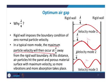
And we have the same explanation that when the panel is being used within a closed room, then the modes of the rooms have generated like this that at every lambda by 4 the particle velocity is the maximum. So, what happens is that the maximum particle velocity occurs at lambda by 4 whenever the modes are set up within a room and because the maximum particle velocity is here.
