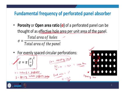
So, here we define how to define the perforations of a cavity. So, there should be some terminology by which we can say this is how the panel is being perforated. So, the very common terminology that is used is called as an open area ratio or porosity.
