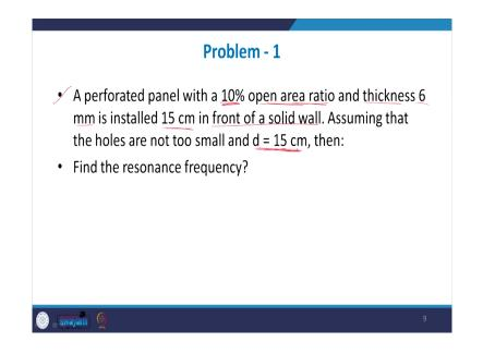
So, we have a perforated panel is given to us 10 percent is the open area ratio and thickness is given as 6 millimeters and it is installed 15 centimeters in front of a solid wall.
