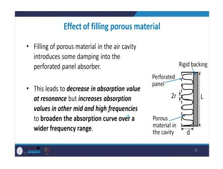
So, what is the effect of the porous material is that we know that such kind of resonators, they only work in a selective frequency. So, as soon as the resonance hits suddenly alpha will jump.
