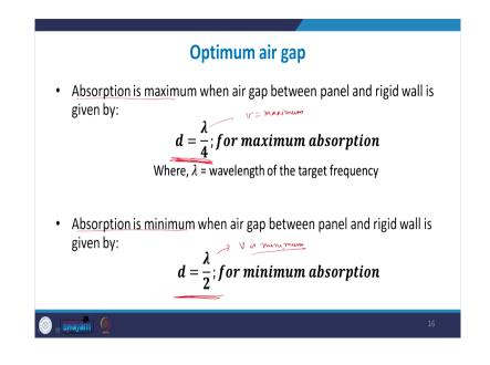
So, now that we have solved two different problems based on perforated panel. So, it gives us a better understanding. So, just like in the case of panel resonators, there was an optimum air depth at which maximum absorption took place and an optimum depth at which minimum absorption took place exactly the same rationale here. So, the absorption will be maximum at the when the cavity depth is lambda by 4 and the absorption will be minimum and cavity depth is lambda by 2. (Refer Slide Time: 25:00)
