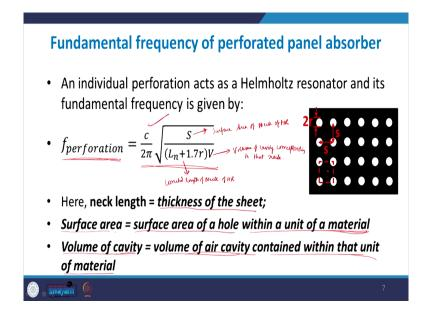
For a Helmholtz resonator, this was the fundamental frequency c by 2 pi into S. Here S was the surface area of the panel of the resonator; let us say. So, it was the surface area of the neck and this was the corrected length of the neck; so, of the neck of the resonator. So, this was for a Helmholtz resonator and this was the volume of cavity corresponding to that Helmholtz corresponding to that neck.
