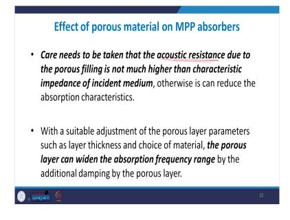
So, in that case; so in that case the acoustic material it acts has many the porous material will give a more resistance. So, overall the effect will be that add the resonance, the MPP will have large loss due to absorption, but if you add the porous material; then it will offer some resistance to air flow. So, it will offer some resistance to the resonance oscillations.
