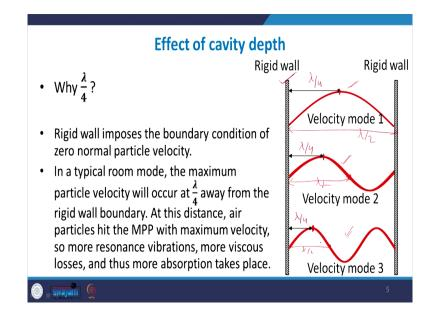
So, this is the explanation here. So, when the perforated panel is used indoors in a closed room, so there is going to be a boundary between the rigid walls. So, whenever the; so this shows us the various velocity modes that are set up with this rigid wall boundary.
