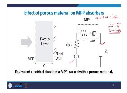
And when you choose a carefully chosen value then the electrical circuit for this value becomes; let us see we have a source here and this is the resistance and the reactants of the MPP. So, porous material add the; add just filled up the porous material just behind the MPP sort of adds like another series impedance that is being added to this system.
