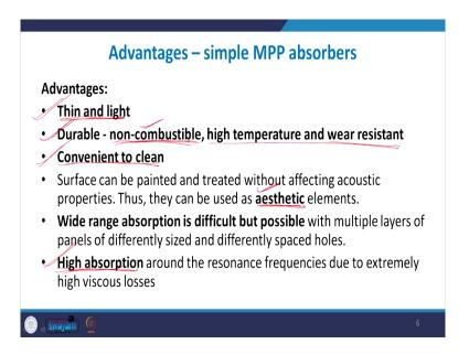
So, what is some of the advantages and limitations of some; some simple MPP absorbers? So, the advantages are pretty clear; so they do not; they are not made up of porous material or fibrous medium, so they are not clean, unclean. They do not need to be maintain time in again to see that all the fibers are properly located, they are not falling apart etcetera. So, they do not contaminate the machine re component or wherever they are used; so they are; obviously, convenient to clean.
