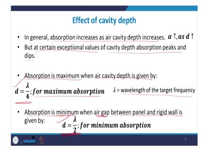
So, what is the effect of cavity depth? As you already saw, as you increase the cavity depth; absorption is going to increase, but absorption will increase with increase in cavity depth. But at some certain exceptional values; the cavity depth absorption will peak and dip. So, although in general for most all the remaining values as d increases, alpha will increase, but at certain
