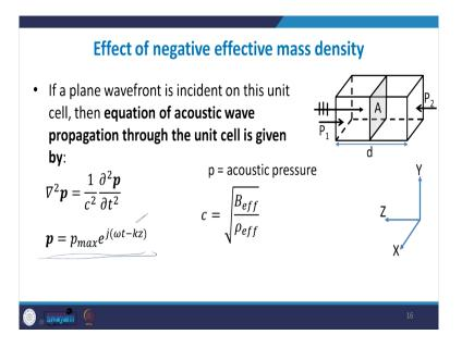
Now, we know that when a plane wave front is incident then the it is given by this equation here each of the p max into e to the power minus j omega t minus k times of z and c is equal to b by rho.
