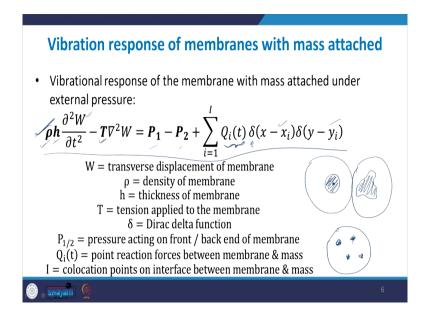
Now, the vibration response of this particular, so, whenever you have a membrane with some mass attached on it then the vibration response of that membrane is given by this particular expression here, if you can see. So, the derivation of this expression is obviously, not something within the scope of this course, you can do you can do that as a you can try it at home if you want to, but it is not a part of the course.
