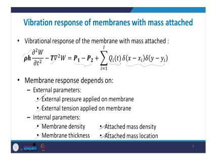
So, overall what you get is that this response it depends upon some external parameters like the external pressure applied which is this, the external tension applied which is this and some internal parameters which is the membrane density thickness and the attached mass density, now this particular point reaction. So, this is the reaction force due to every point mass within the total mass. So, we have we are considering this total mass as a collection or a continuum of many point masses.
