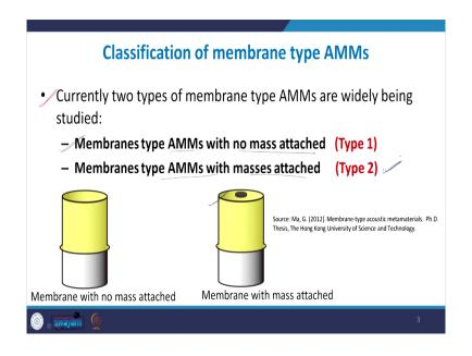
So, here just a revision quick revision again of the, so, as you can see here. So, you have 2 types of unit cells: the first one is the membrane type AMM with no mass attached and the other one is with mass attached and this is what we will discuss today in this particular lecture.
