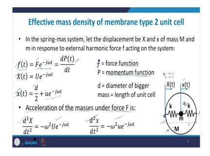
So, let us start with the derivation for effective mass density for the type 2 unit cell. So, in this case let us say, now let us see we are taking this equivalent mass spring model for the unit cell. So, let capital X t bt displacement for the bigger mass M and small x t be the displacement for this smaller mass small m. If we take the origin here, so, this is where X begins. So, X or the displacement begins from here this is the point where this begins.
