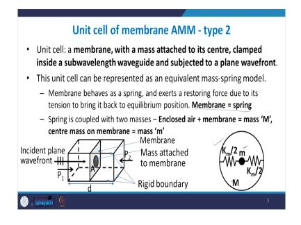
So, the unit cell is effectively it is a membrane with a mass attached and at the center and it is clamped inside a waveguide and subjected to a plane wave front. So, this just like the previous unit cell, this can also be represented by an equivalent mass spring model. So, in this case what happens is that here when the vibration when the air vibrates, the membrane is going to be the spring element because that is the only element.
