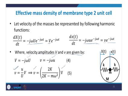
Now, let us find out the velocity functions. So, we have X we differentiate it once with respect to time. So, this becomes the first velocity function for the bigger mass and for the second mass this is the velocity function which we can represent as some amplitude into e to the power minus j omega t and some velocity amplitude into again e to the power minus j omega t.
