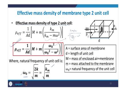
So, we have got an expression for the effective mass density of the type 2 unit cell. So, here A is the surface area of the membrane, d is the length of the unit cell, capital M means the mass of the enclosed air plus the membrane. So, both air and membrane together what is their mass and small m is the mass attached to the membrane.
