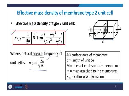
So, if you see here rho effective is this particular expression here. So, here in the here this is 1 by A into d; here A is the surface area of the membrane, d is the length of the unit cell. So, A actually is the surface area of the membrane when the membrane is not being transferred when the membrane is in equilibrium, it has not undergone any transverse displacement.
