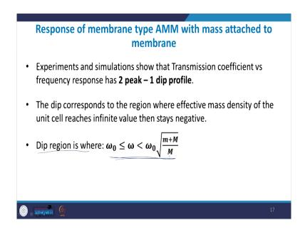
So, to summarize from both the experiments and simulations so, what we see is that, when we use this kind of metamaterial, then the transmission versus frequency response is actually a two peak one dip profile and the dip corresponds to the region where the effective density becomes negative. So, the dip region is where this is being satisfied.
