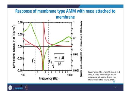
So, this is for the same material this is the graph of the effective density. So, as you can see the same point where you obtained a heavy dip in transmission, it corresponds to the point where you have the region of negative density.
