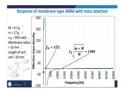
So, let us do an exercise here. So, I have plotted how the rho effective varies with the variation in the frequency. So, the parameters I have taken is that, I took a membrane its a light membrane whose mass is 0.2 grams and the smaller mass the smaller dense mass which is attached on top of the membrane, it is 17 grams. And the unit cell is such that omega naught is equal to 950 radians per second and omega naught we know is under root of km by m.
