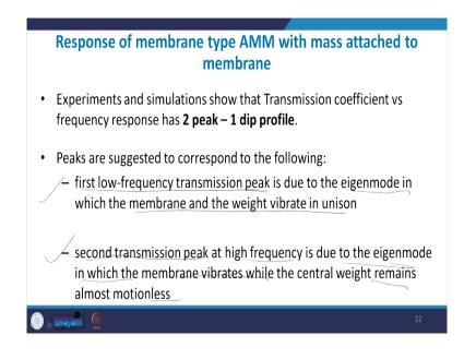
So, transmission versus frequency is a two peak one dip profile and the first peak is due to the eigenmode where membrane and the weight attached to it the both oxalate in unison, they are coupled together. And the second one corresponds to the eigenmodes where the membrane is
