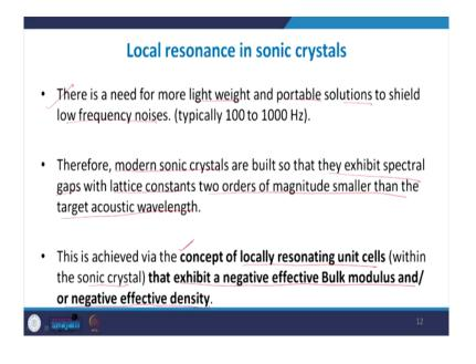
And that is why some sonic crystals have been created which operate on one additional principle. So, that will be the principle of local resonance and the creation of negative effective elastic properties.
