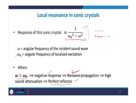
Now, the response of this particular sonic crystal was is almost directly proportional to this quantity here. So, when we solve some numerical; you will get a better idea on how the various sonic crystals work. So, here the response of this crystal is given by this expression here where this is the angular frequency of incident sound wave and this is the angular frequency of localized excitation.
