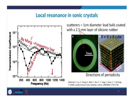
So, if you another way of representing the response of this structure is as a transmission coefficient by frequency. So, as you can see that mass frequency laws states that as the frequency increases, the noise reduction is going to increase or the transmission coefficient is going to go down because of low transmission. So, transmission coefficient should go down with the increase in the frequency.
