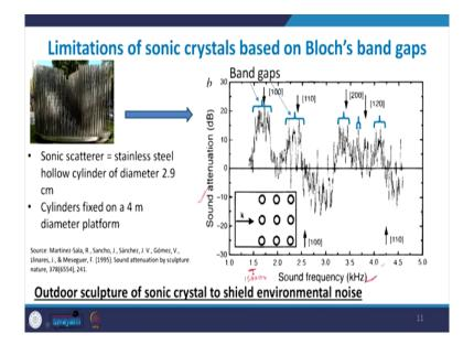
This is the typical response; so here we have the sound frequency in kilohertz and the sound attenuation in decibels.
