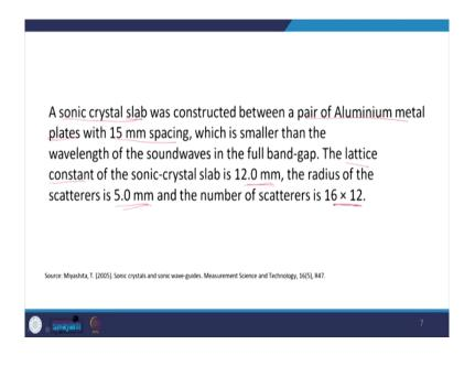
So, this is some of the specification. So, the slab was the sonic crystal slab was created between a pair of aluminum metal plates 15 millimeter spacing. So, definitely all the dimensions were kept smaller than what is the target frequency, to satisfy the Bloch's theorem. And the lattice constant is given to be 12 millimeters, the radius of the scatters is 5 millimeters and they are arranged in a 16 cross 12 format.
