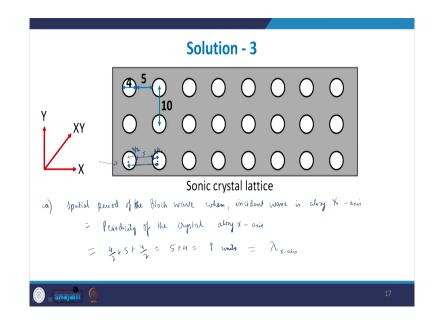
So, let me rewrite this phrase here. So, here the spatial period of the Bloch wave when incident wave, the wave that is incident on the crystal is along X axis. This period will be same as what is the periodicity of the crystal along X axis, plane wave front is incident here as we know and a plane wave front will create harmonic plane waves inside the crystal. And, the direction of propagation will be the same provided this crystal does not create bending.
