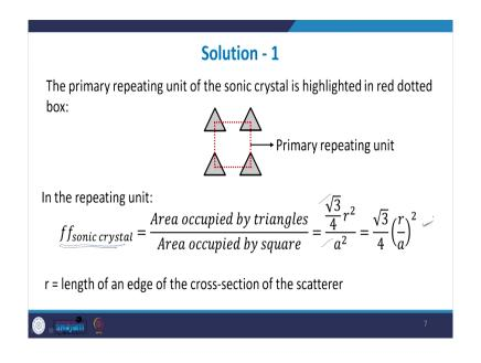
So, the overall filling fraction for the sonic crystal is what? It is the area occupied by the triangle divided by area occupied by the square within the repeating unit. So, when you do this, this is the expression you end up with; here r being the length of the edge of the cross section of the scatterer.
