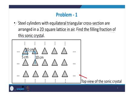
So, here we are given steel cylinders are being arranged; so, we have a steel cylinder. So, this gives our top view of the sonic crystal. So, otherwise they are cylinders and they have an equilateral triangular cross section. So, this is the cross section of these steel cylinders, they
