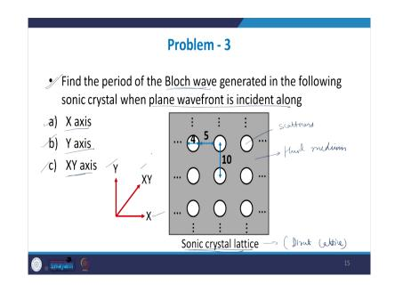
So, the third question here is given is for Bloch's theorem. So, let us say this is the question here. So, again we have some sonic crystal lattice, now this is actually a direct lattice, this is not a reciprocal lattice and I have to what; so, this is the sort of arrangement. So, here these are the various scatterers and this is the fluid medium and this is how the sonic scatterers are arranged or some metals, the metal rods are arranged.
