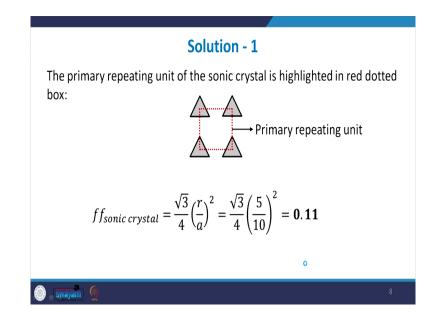
So, this is what you have end up with and we know that this r is given to us is 5 and a is 10. So, if I go back to the question just one more time. So, here this is 5 centimeters, the side length of a triangle and for the square it is 10 centimeters. So, when you put that value here in this expression it is root 3 by 4 into 5 by 10 whole square. So, this is what you get; so, this becomes the filling fraction. So, this is the end result.
