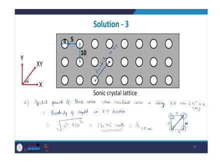
So, again what so, what I can write here is that this XY axis is actually 45 degrees to this horizontal axis here; so, this is the called as the XY axis. So, it will be equal to what is the period or the periodicity of the crystal in this particular direction and how do we solve it? So, here let me take this particular case here. So, this is how the arrangement is and this distance here is 9 and this distance is 10; so, I will just write 10 here.
