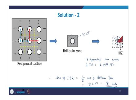
So, what we see here is that, this was the square and the area of this is 84 64 units is the total area of the square. Now, to reduce this further and remove all the symmetry an IBZ has been drawn and if you can see here, if you draw these lines like these so, this is how I have drawn the lines. So obviously, then this is 1 IBZ and this portion is symmetrical to this above portion. So, this is the second one and this portion is symmetrical to this one, this is symmetrical to this, this and this.
