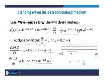
So, let us use this condition. So, the pressure let us assume a general pressure equation for the wave inside this long tube. Now, inside this long tube because, here the lateral dimension we have assumed to be very small the tube is very long so, the length is very long. So, in that case the waves generated are only harmonic waves.
