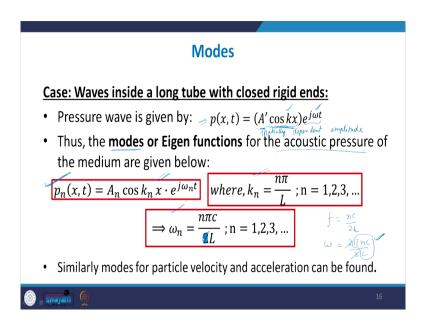
So, this is the pressure wave here I have just used, I have replaced this twice a with another constant a dash so, it is some constant a dash times cos k x; this is the spatially dependent amplitude and this is the time varying function. So, we are getting a pressure wave solution.
