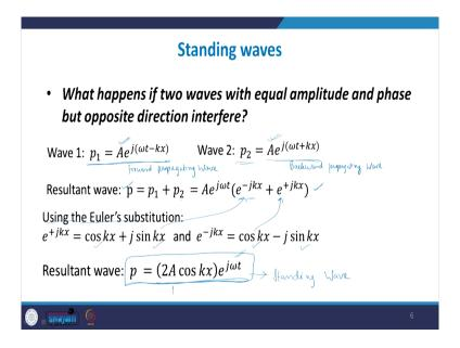
So, let us study this case. So, let us say we have wave 1 and the pressure of that wave is given as Ae to the power j omega t minus k x and the wave 2 is given as Ae to the power j omega t plus k x. So, as you can see here both of them have the same amplitude, there is no phase difference and 1 is propagating forward so, this is the forward propagating wave and, this is the backward propagating wave. So, they both are traveling in the opposite direction with equal amplitude and phase.
