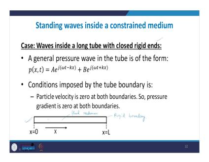
Let us study the second case, which is when the waves are generated inside the long tube with closed rigid end. So, now, we are taking the case of a constraint medium. So, here there is a constraint which means, that the medium has got fixed boundaries. So, the waves are being generated in a long tube with a closed rigid end. So, let us see here; so, waves this represents fluid medium, in this particular figure and all this is the rigid boundary. So, this is a constrained medium.
