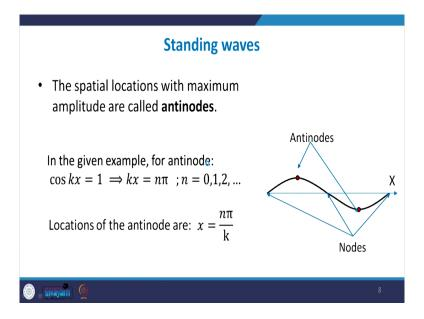
So, let us find out, where are the different terminologies here? So, in a standing wave you see that there are certain points where the amplitude reaches a maximum value. So, in this particular animation, these red dots these red dots are the places where the amplitude is the maximum and these are called as the antinodes, the red dot places.
