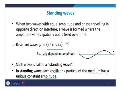
So, this is a animation again and this is our resultant wave, that we have found. So, here the amplitude it is spatially dependent. So, for difference for different X locations the amplitude is different, but it is fixed and there is a sinusoidal motion with respect to time, and such
