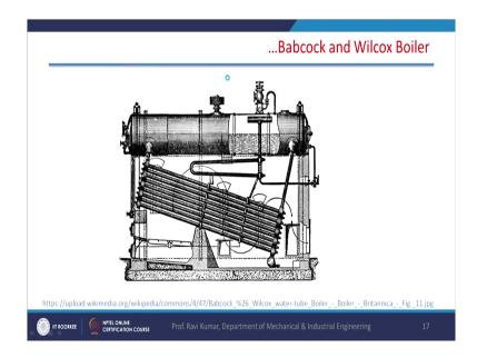
This is the schematic of the boiler; you can see these tubes are inclined there are inclined at a degree 10 to 15 degree. And, there is a super heater which is taking steam from here and steam is circulated in the super heater and this steam after coming from here it goes through the.
