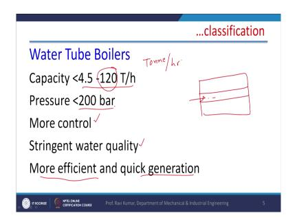
Now, this is about water tube boiler capacity it can go up to 120 tones per hour steam this is steam generation capacity 120 tones T o double n tones per hour. That is the steam generation capacity of the boiler this is the range 4.5 to 120. Pressure; it can go up to 200 bar right controls more controls are required. Because, the water is flowing inside the tube suppose there is a obstruction in the flow of water then accident may take place right.
