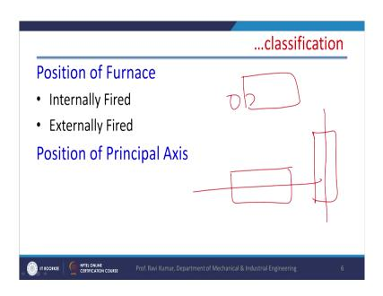
Position of furnace; that is another way of classifying the boilers whereas, boiler is internally fired or it means the furnace is housed inside the boiler or it is outside the boiler. So, there can be a I mean number of classification position of principle axis the boilers are is a horizontal, it means the principle axis is horizontal, boiler is vertical principle axis is vertical.
