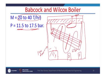
So,. So, in the largest boiler, it produce I mean capacity of this boiler is 20 to 40 tones per hour and pressure also can vary between 11.5 to v 17.5 bar and this is a water tube boiler it is not a fire tube boiler.
