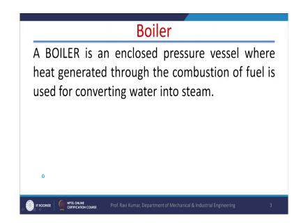
Now, what is a Boiler? The boiler is an enclosed pressure vessel where heat is generated through the combustion of fuel and this heat is used in conversion of water into the steam. So, primarily the boiler is enclosed vessel and the main purpose of the boiler is to generate a steam higher the pressure more work extraction from the steam.
