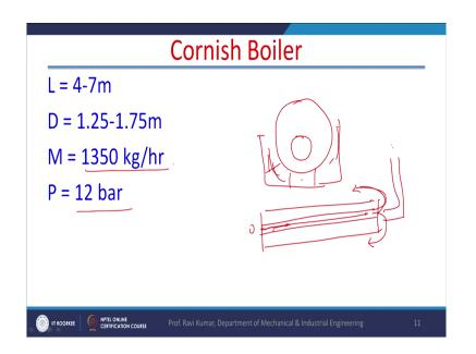
So, after the lancashire boiler we will discuss the cornish boiler. So, cornish boiler is smaller in size. So, here the length is varying between 4 to 7 meters diameter of the drum is 1.25 to 1.75. So, it is smaller in size and it has only one tube that is the difference between lancashire boiler and cornish boiler. And this tube is also centric it is not centrally placed right.
