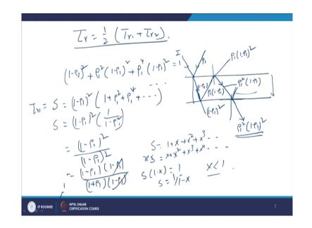
Now, transmissivity is also average of both the components. Now suppose on a plate let us assume there is a plate there is a cover plate there is this incident of light I reflected rho I. So, the light which is entering the cover plate is entering the cover plate is 1 minus rho 1 right. Now this 1 minus rho 1 light intensity of the light will again reflected from the bottom of the plate. So, it is going to be the rho 1 1 minus rho 1 right.
