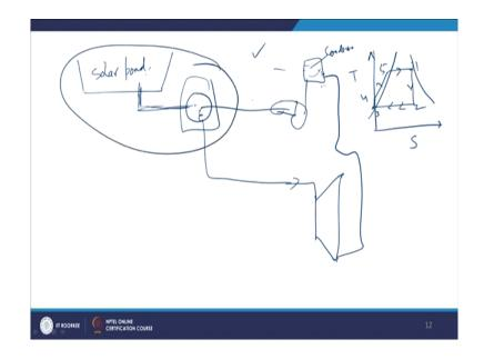
Now, for the low power generation, there is a system which is known as solar pond which is normally used for solar thermal energy storage. So, from the solar pond, there is normally brain it is the salt is mixed in the solar pond. So, there is a the brain and the brain can go to the heat exchanger because power generation method is same the Rankine cycle; the thing is how we get the steam out of the feed water. So, the power generation processes is same old Rankine cycle.
