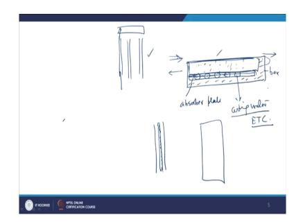
So, flat plate collector has a box there is a box, it is very simple in construction it can be a wooden box or a metallic box or nowadays pvc box are also available. Now, this box has an absorber plate this is a box and this box haves has absorber plate this is absorber plate.
