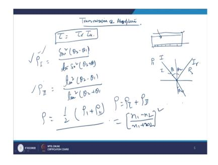
Now, the where from the energy is coming in the collectors it is coming from the plate transmission plate cover plate right and it is coming in two forms. First of all transmission energy to the absorber by transmission an absorption there are two ways. Now, total energy transmitted is total energy by transmission total and total energy by absorption that is total energy coming to the plate.
