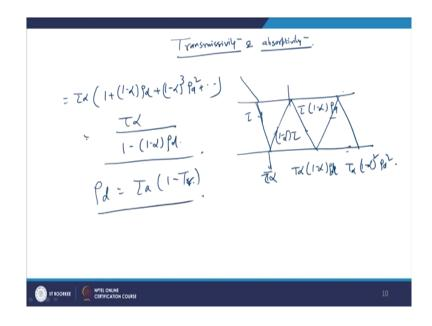
So, transmissivity we have to these for the absorption transmissivity calculations and absorptivity calculation right. If you take both into the account, suppose now we take the glass amount of radiation is transmitted, after transmission it is absorbed right. This is reflected right and it is going up and then again when it is going down it is this is due to reflection.
