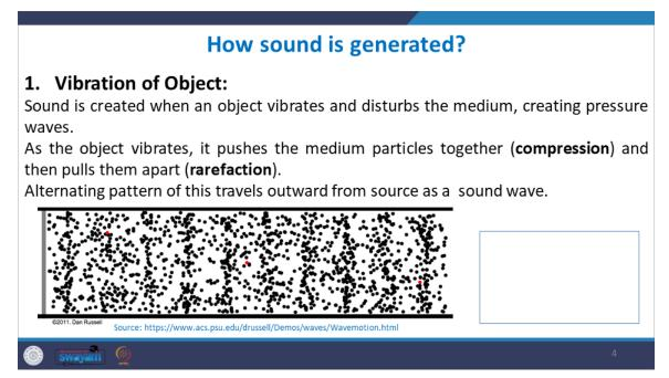
gray thing here which is a piston and this piston is inside a pipe and as it is moving back and forth the particles of the air or the medium they are coming together and the moment they come together they increase the pressure slightly. The moment they go away again, they decrease the pressure. And this particular disturbance of fluctuation in the moment instantaneous pressure is carrying forward as the sound wave.
