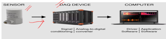
DAQ block diagram and elements of modern digital DAQ
