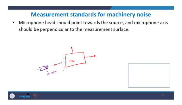
So, another thing you have to ensure is that the microphone head should be pointing towards the source, and the axis should be perpendicular to the measurement surface. suppose you have machinery here which is radiating noise in whatever possible directions, you should ensure that your microphone is pointing like this. This is your microphone head. It is pointing directly towards the machinery, perpendicular, and the axis here is perpendicular to this measurement surface.
