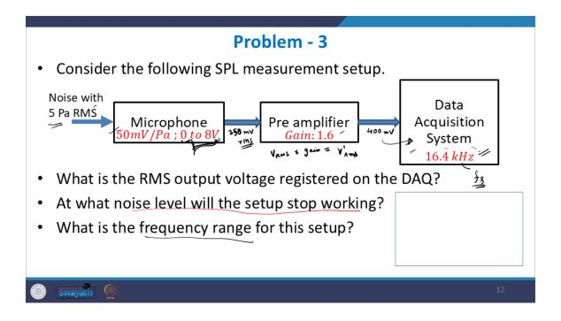
So let us solve another problem. We are given some recording setup. We are recording the sound pressure level. some noise whose PRMS is 5 pascals is incident on a microphone, and some kind of values are given for this microphone.
