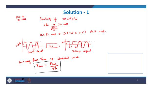
Here let us see it has a sensitivity of 20 microvolts per Pascal. which means that if 1 Pascal of sound pressure is passed, be it an RMS pressure and amplitude, just the value of 1 Pascal of acoustic pressure, it will create 20 microvolts of voltage when it is passed through this mic A. 1 Pascal input, 20 microvolts is the output. In that case, if you think about it, 0.5 Pascals amplitude should give 20 microvolts multiplied by 0.5 as the voltage amplitude.
