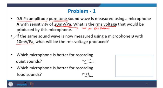
the first part of this problem. So over here, it is given that the microphone here 0.5 Pascals amplitude is being passed to it, and the sensitivity is 20 microvolts per Pascal. for the mic A, what it essentially means is that all these sensitivities are measured for microvolts per RMS pressure that is passed to it.
