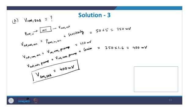
What we have to find is the VRMS at DAQ. here, what does the microphone do? The microphone converts this PRMS, whatever is input into the microphone, into some RMS voltage. Let us indicate the input and the output for the microphone using the subscript mic or the subscript mic. Then the V output RMS from the microphone should be simply whatever is the pressure.
