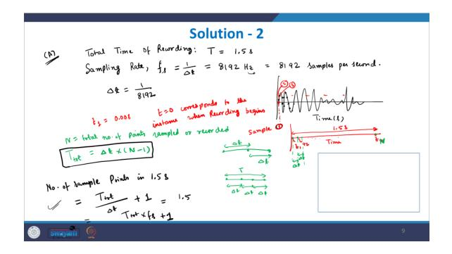
Here we are given that, the total time of recording t is 1.5 seconds, and we know that the sampling rate is inversely proportional to the sampling increment or the time interval between any two samples.
