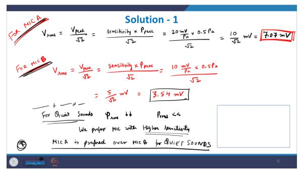
What you get ultimately is that the RMS voltage that is obtained would be the peak voltage by root 2,
