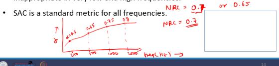
OK, so let us now see the second measure used for evaluating the sound absorption by a material. So here, the first measure was SAC, but SAC is not a single-value measure, OK? You see, it is a variation with respect to frequency, but as a noise control engineer or any engineer, we are always fascinated with having some single-value measure just for a very quick analysis and estimate. So, that single-value measure here becomes, you know, the noise reduction coefficient, OK. So, what is it?
