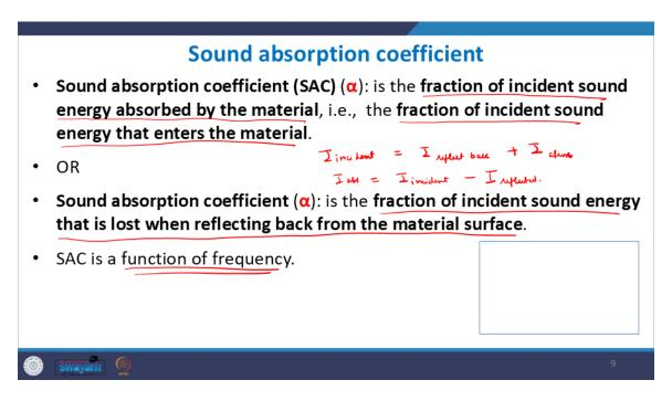
It is the fraction. So, if you see here, this is the fraction of the incident sound energy absorbed by the material, i.e. the fraction of incident sound energy that is entering inside the material, okay. So, what is so if, suppose, a 1 pascal sound wave is incident—intensity of 1 of sound wave is incident—how much of it is actually going into the material without reflection? So, the fraction of incident energy that is getting absorbed or entering the material.
