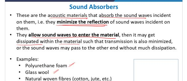
How do you minimize the reflection? So, whenever the sound wave is hitting a material, you minimize it because you do not want it to reflect back. So, basically you would like it to pass through. So, these materials allow the sound waves which are incident to enter inside it. And once they enter inside it,
