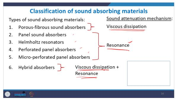
So, for porous fibrous sound absorbers, we have viscous dissipation that happens. For these other absorbers—panel, Helmholtz, perforated panel, and micro-perforated panel—the resonance phenomenon leads to sound attenuation.
