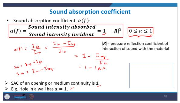
Okay. So, the sound absorption coefficient is a function of frequency. It is defined as the sound intensity that is absorbed by the material divided by the sound intensity that was incident on it, and it is 1 minus mod r whole square, okay.
