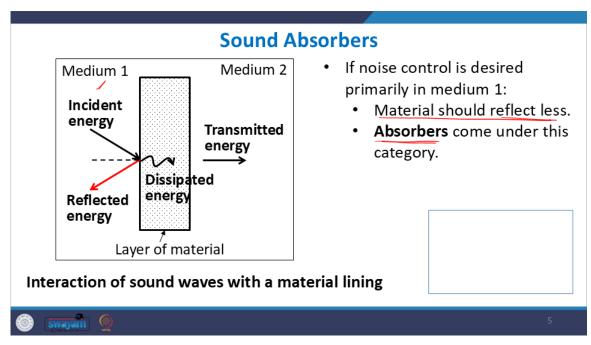
incidence or near the source so absorbers fall under that category where the materials they have to minimize the reflection okay so how do we define them these are the acoustic materials that absorb the sound waves whatever is incident on them that is they minimize the reflection of the sound waves So, how do they do this?
