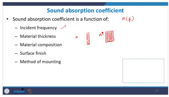
So, the sound absorption coefficient, the measure first of all, is a per unit area measure without any units. And it is a function of, you know, what frequency is being incident, as I told you that alpha is a function of frequency, OK. It also depends on the material thickness because this is a per unit area quantity.
