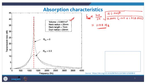
It is C0 let us take it as 340 at room temperature by 2 pi and you have this S here S by V into L plus 1.7 r. So, S is the cross sectional surface area of the neck. So the neck radius is given assuming a cylindrical neck. If nothing is given you assume it is a cylindrical neck. So pi times of this pi r square should give you the cross sectional area of the neck. The volume of the cavity in the SI unit is given as this and then within that you have L plus 1.7r. So, the length is 7 millimeters.
