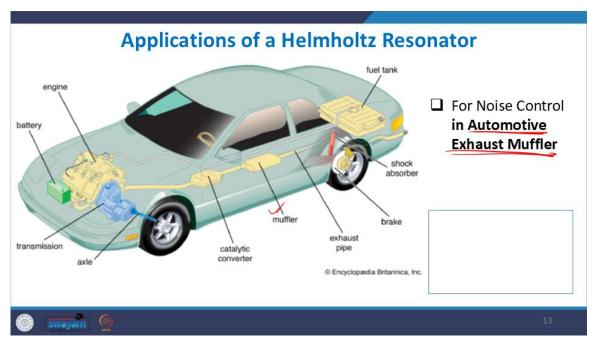
A Helmholtz resonator is there in every modern automotive exhaust muffler. So, it is very widely used in this application. So, what is the purpose to reduce the exhaust noise? You can see here in this vehicle you know. the muffler is there in the tail pipe or the pathway of the exhaust.
