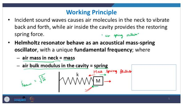
the incident sound waves hitting. So, from the outside environment, suppose there is some noise source which is creating these pressure fluctuations or sound waves. Which hit the neck, and when they hit the neck, they can create vibrations in the molecules of the neck.
