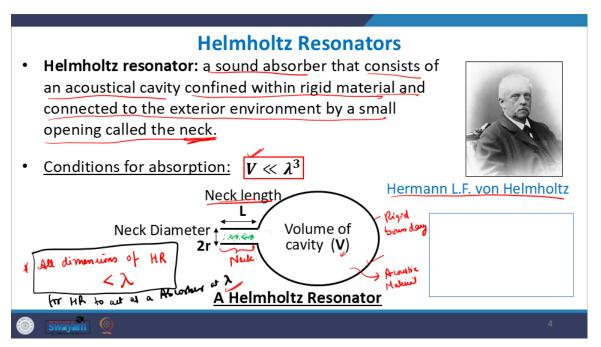
It was proposed by the scientist Hermann L. F. von Helmholtz, and it is named after him. So, this is a sound absorber. It consists of an acoustical cavity which is confined within some rigid material or some rigid boundaries. and then it is connected to the exterior environment by a small opening called the neck. Ok. So, it looks something like this.
