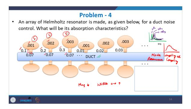
So, for  $HR_1$  what is the fundamental frequency for this one let us say we put the various values. So, we have been given these various dimensions this is the volume of the cavity this is the neck of the this is the length of the neck ok and this is the diameter of the neck. So, these values are given for the different Helmholtz resonators. So, you can put it and find out the value.
