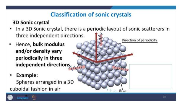
And then the steel and air gap, and so on. So, this is happening in this direction, and there is a periodic layout in 3D. So, even here in this direction, periodically, the properties keep changing. When the sound waves are propagating, okay? So, the red zone indicates the beta rho for the steel, and the yellow zone indicates the beta rho for the air medium, and so on.
