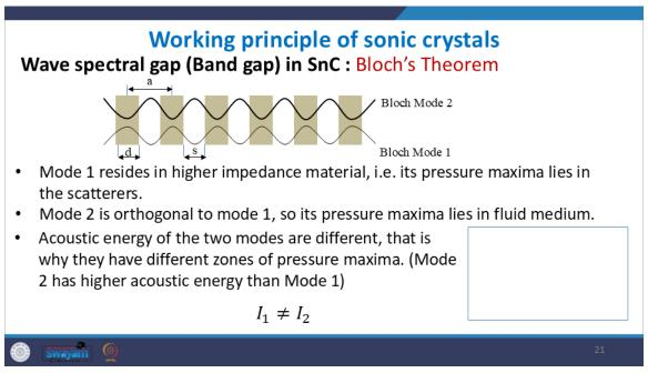
A more acoustically dense region occurs for a lower mode. So, here As you can see by the nature of this, mode 2 is higher because here the pressure maxima occurs in a lighter region, and in mode 2, the pressure maxima occurs in a denser region. So, these two modes have different acoustic intensities, and you know that acoustic intensity is what? For a plane wave propagation, it is p squared by rho c.
