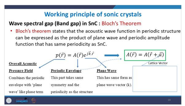
So, suppose We are considering a sonic crystal that has some periodicity of A, which means that the B and rho are changing after every distance a. Then the amplitude of the wave will also be periodic in nature and will change with every distance a. Okay. And because it is a plane-propagating wave, the nature of propagation will be maintained as a plane-propagating wave. But the overall amplitude will be periodically varying with the periodicity of the structure.
