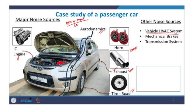
You can see that obviously, if you open the bonnet, you can see the engine that is operating. The internal combustion engine is a major noise source.
