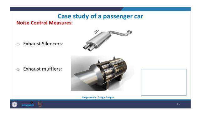
Inside, as you can see, these are the perforated components. Then you have the Helmholtz resonator cavities, and based on these perforations and resonance phenomena, it is able to absorb the noise. The purpose is to absorb the noise and reduce the back pressure.
