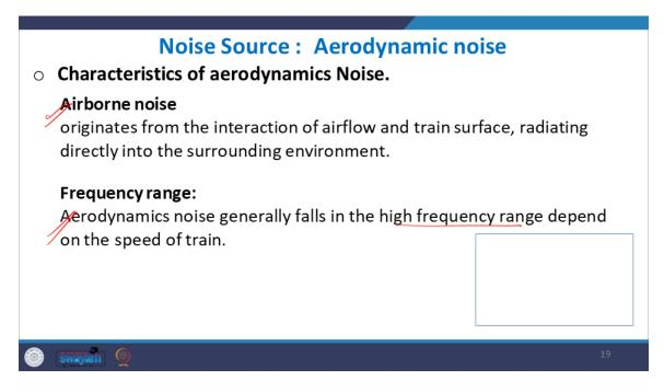
What are the typical frequency ranges? The aerodynamic noise generally falls in the high-frequency range, depending on the speed of the train. What are the strategies that we can adopt to mitigate this aerodynamic noise? So, we need to reduce the turbulence that might be caused when the air flows over the body. And hence, a more streamlined design is required.
