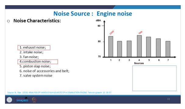
Now, what is the impact of this engine noise? High-level airborne engine noise can propagate into the train cabin.
