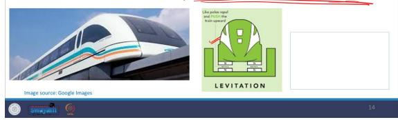
This is a new form of train propulsion technology where the train moves using electromagnetic induction. So, many of the tracks have electromagnets. Due to the attraction and repulsion between the train's electromagnets and the track's electromagnets, the train moves forward. So, what happens here is that the train is never in contact with the track. There are no wheels on the train and no traditional railway tracks.
