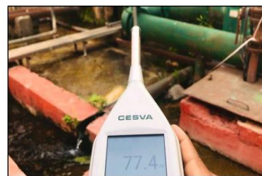
SPL of Cooling tower (77.4 dB-Z)
