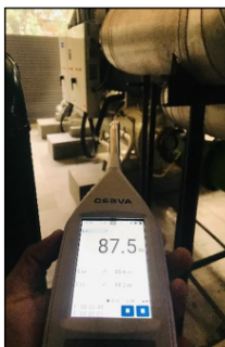
SPL at single chiller operating condition (87.5 dB - Z weighting)
