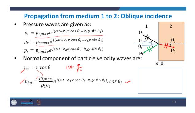
Now, once again, have a look at these equations. We have these equations for pressure. Now, let us find out the equations for the normal component of the particle velocity at the medium.
