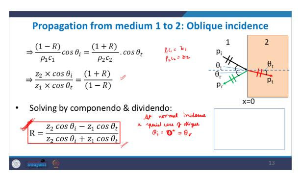
If you take that this is a generic equation, and normal incidence becomes a special case of this generic equation. So, at normal incidence, which is one particular normal incidence, a special case of oblique incidence. So, for this generic case,
