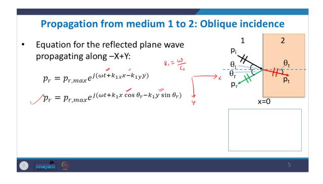
reflected wave? It is traveling in the positive y but the negative x direction. So, that is why we have a plus sign in the x component and a minus sign in the y. If you again resolve this and write it in terms of k1, and here, because the reflected and incident waves are in the same medium, they both have the same wave number k1, which is
