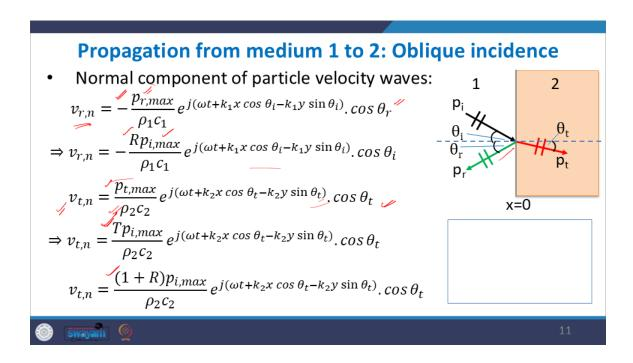
In the same way, we can find out the normal component of the reflected wave. So, once again, we use the equation of the reflected wave. We divide it by  $\rho_1 c_1$  for that medium and then multiply by  $\cos\theta_r$ , and then we place a minus sign here because the wave is propagating like this. So, if you resolve and find out the normal component along the x-axis, the wave is actually propagating along the negative x-axis. So, the normal component is opposite in direction.
