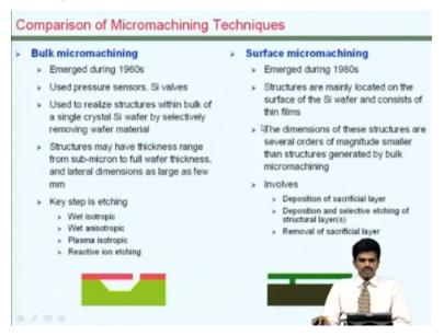
As you could see from here, in surface micro-machining you are essentially adding a small component to the surface of the silicon wafer, whereas we dig into the wafer itself in the case of bulk micro-machining. Various components have been demonstrated using both these techniques and have become the main stay in building microsystems. So both surface and bulk micromachining techniques are important. Thank you very much.
