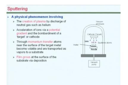
We will see these in subsequent slides. One of the physical methods is known as sputtering. In sputtering, we create a plasma with a neutral gas and these ions that are formed will hit the cathode and we keep the target at the cathode so that the incident ions would displaces atoms from the target which is essentially the source material in this case and the sputtered atoms from the target would be made to deposit or stick on to the wafer which is kept at the anode.
