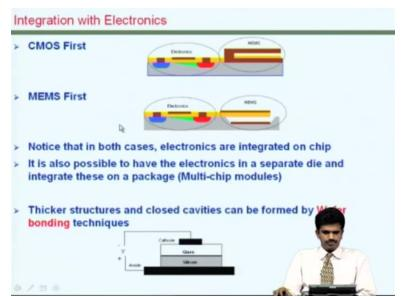
As in surface micro-machined structures, bulk micro-machine structures can also be integrated with electronics. This could be integrated on chip or even at the package level as multichip modules, but in micro-machining, you can only have cavities as deep as the wafer thickness. When we want really thicker geometries, we want to look at possibilities of bonding multiple wafers and processing them further.
