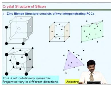
In the context of the silicon wafer which is essentially a zinc blende structure consisting of 2 interpenetrating FCCs. If you recall, this is 1-unit cell of that with dimension here which is the
