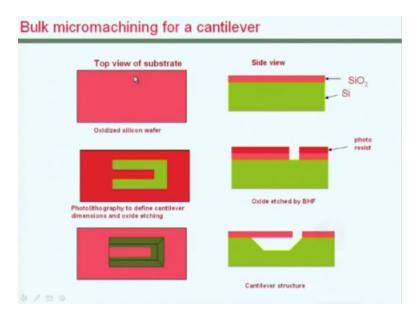
What happens while etching is that when we form this surface, let us say we use oxide as the etch window film and create this cavity, the hole here in the etch window but as etch progresses what would happen is that 111 plane will get formed here as well as here. It will get formed here, it may get formed here, here on this side as well as on the side below the protruding parts. But the diagonal line here from this convex etch, the atoms on that side will not be as stable.
