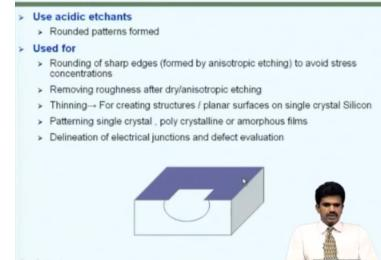
As I mentioned, one of the simplest thing to imagine would be the isotropic etching usually done by using acidic etchants and results in rounded patterns as you could see from here and these shapes are usually unpredictable and dependents largely on the agitation and various other process parameters. Isotropic etching is also used when rounding of sharp edges are actually required. This is typically required to avoid stress concentrations.
