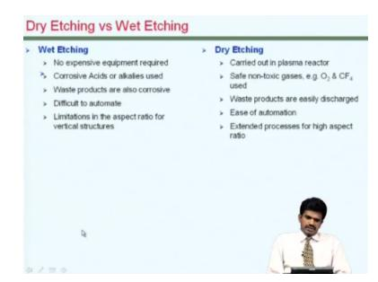
Compared to wet etching, this kind of dry etching is usually far more expensive. We need to carry out these reactions in a plasma reactor which obviously at the low pressure and hence all the additional equipment required for that purpose. We use corrosive acids and alkalies for that etching whereas we can live with oxygen, carbon tetra fluoride and other non-toxic gases for etching in the dry phase.
