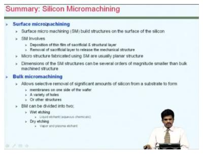
Compared to surface micro-machining, bulk micro-machining allows removal of significant amount of materials and hence larger structures are possible. In both surface and bulk micromachining, dry and wet etching are utilized effectively. The dimensions of structures formed by surface micro-machining, can be several orders of magnitude smaller than in bulk material and but can have very large dimensions and very thin vertical dimensions.
