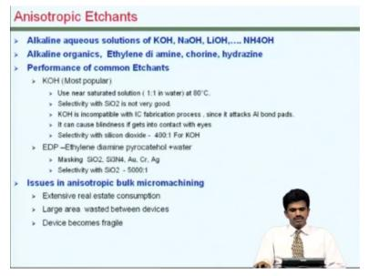
Etchants used in an isotropic etching are usually alkaline aqueous solutions. KOH is by far the most popular material and it has reasonable selectivity with SIO2, better with silicon nitride. The selectivity with silicon dioxide is of the order of 400:1. Another chemical which is used for etching silicon is known as EDP (ethylenediamine pyrocatechol) which is aqueous solution of this.
