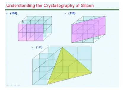
For a quick overview, we can look at how Crystalline structures are defined. 100 surfaces are in which the wafer surface is aligned to any of coordinate directions with respect to the lattice arrangement. In 110, the surface is diagonal with respect to 2 of the access whereas parallel with respect to one of the third. In 111, the surface of the crystal or the resulting plane is inclined with respect to all the 3 crystal directions.
