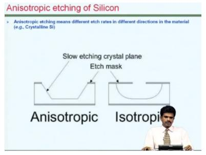
Anisotropic etching on the other hand make use of the crystalline nature of silicon in realising well defined geometry. As see from here compared to the isotropic etching which results in rounded geometries and also what is known as undercut which is essentially etching beneath the etch mask geometry. In anisotropic etching, if the geometries are decided well, we can ensure that there is minimal or no undercut and a continuous plane which would form the etch profile.
