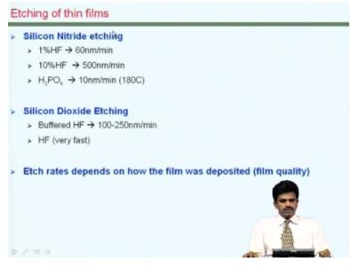
Etching of thin films of silicon nitride can be done usually using phosphoric acid. Silicon dioxide can be done using the etch of solutions. It may appear that the silicon nitride has lower or comparable etch rate as silicon dioxide, but it so happens that the nitrate films are usually thinner
