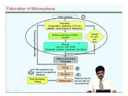
Obviously, the steps involved are very similar to the overall process flow. The constituent steps include deposition pattern transfer and etch, and in this case various standard lengthened etching steps are required to form the cavities on silicon. So, the emphasis here is on itching itself. **(Refer Slide Time: 06:55)**
