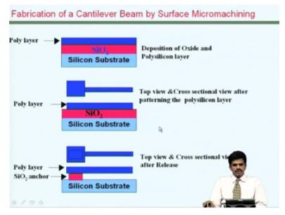
On the other hand, when thin microstructures are required, we look for surface micro-machining. In this example, cantilever structures are formed where poly silicon is used as a structural material and silicon dioxide can be used as the sacrificial material.
