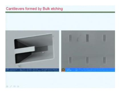
So, what is critical is that these edges are aligned with respect to the 110 directions on the surface of the silicon wafer. So, this gives you significant reason in aligning the geometries with respect to the crystal orientation of the silicon wafer.
