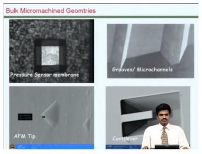
By bulk micromachining because you are basically etching into the bulk of the silicon wafer. We can form diaphragms or cavities as you see here, grooves or channels as you see here or we could even form cantilever structures like this freestanding above a large cavity. We can also suitably modify the processes required and form tips pyramidal geometries, conical geometries that could be used for applications such as AFM tips. All these are possible by bulk micromachining.
