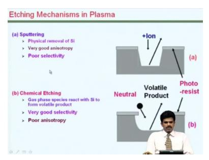
Let us look at the various mechanisms that are possible in plasma etching. If you look at the simple physical removal where only the ion bombardment could be used, there is chance that it is very poorly selected. If you only look at the chemical reactions for the removal of material, it could happen that it is an isotropic.
