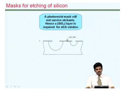
One interesting thing to note at this stage is that the mask material used for defining that etch window is not photoresist as you may have seen in order situations where thin films are etched. The etch process for thin films are fairly quick and during the etching of the thin film, the photoresist that was covering it may not have gone completely, whereas for etching silicon, more powerful etchants are required and usually for a longer time.
