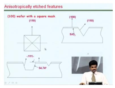
Let us see how this is done in more detail. Depending on the width of the etch window and depending on the duration of the etch we can have either a V-shaped or a widen-shaped cavities, why is it so. It so happens if on a 100 wafer, if you align these rectangular windows properly, the plane that is formed at an angle is 111 plane and in atom in 111 plane of silicon structure are strongly bonded to those underneath them and hence are extremely difficult to be displaced by many reagents.
