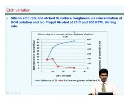
There could be variations based on the composition of the chemical used, the temperature and also the agitation. These variations are usually predictable as long as these parameters are kept within control and hence the anisotropic etching is usually predictable for the overall geometries required.
