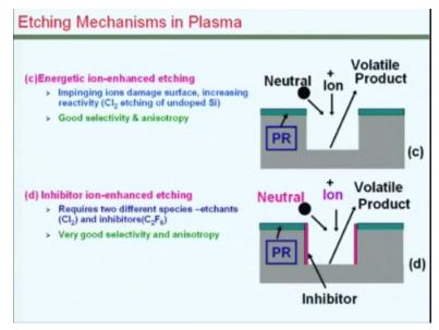
So, we need to have properly energized ions for good selectivity and anisotropy in realizing structures with well-defined profiles. Yet it may become a problem when you want to dig deep into the surface of, dig into the bulk of the wafer. It often requires attaching inhibitors, so that we can have a directionality in going deep into the wafer for deep structures with high aspect ratio.
