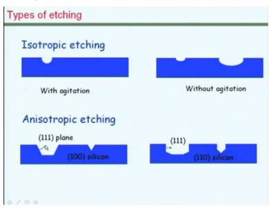
These are explained by the geometries here. What is formed by isotropic etching are usually
