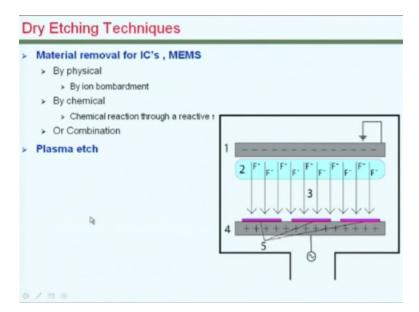
For the successful realisation of micromachining, often dry etching techniques are performed. Dry etching is similar in principle to the sputtering technique that you have seen in the context of deposition. In sputtering if you recall, the ions from the plasma are made to hit the cathode where the target was kept that causes the atoms to get displaced from the target. In the case of etching what we do is instead of the target, we keep the wafer at the cathode.
