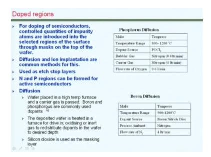
As I mentioned, this would require doping. One of the approaches is based on what is known as diffusion. In diffusion as in ion implantation what is done is that we introduce N and P type materials on to the semiconductor. In diffusion, the wafer is placed in a high temperature furnace and a carrier gas is used which is usually nitrogen to transport boron or phosphorus from the respective source material onto the surface of the wafer.
