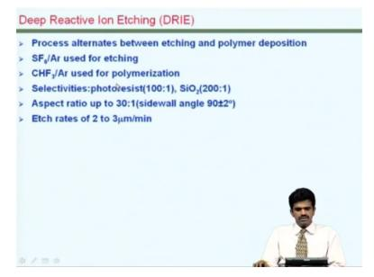
As I mentioned in this, we can use various combination of gases for etching various materials. We also use a step in which the sidewalls are coated with a kind of nonstick polymeric surface. It may go away after sometime, so these removal and attachment processes are cycled, so that high aspect ratio structures are possible.
