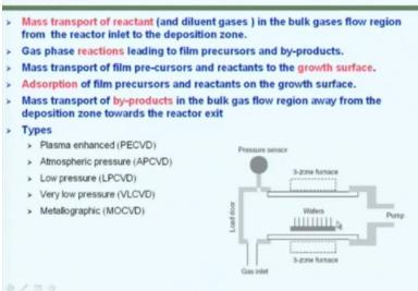
In the chemical vapor deposition on the other hand, the reactant gases are transported into the
