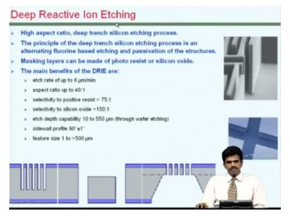
For deep etching of silicon, for forming high aspect ratio geometries, processes known as deep reactive ion itching is required. In this case, what is done usually is that we remove material partially and then do a round of deposition scheme in which the sidewalls would get coated with something like a nonstick surface, so that a subsequent etching when the atoms get displaced, they do not go and stick to the sidewalls. Rather they come out of the cavities.
