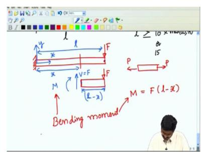
And this we call the bending moment. It is this moment that tries to bend the beam this moment. So that in this particular case will be = this F times L-X that is a bending moment. As we move from this end to that end when we go here L-X. X = L at this point. Let us say this point X = L. So there will be L-X0 no bending moment. As we move towards this bending moment is going to increase as X becomes smaller and smaller as you go from here to here the bending moment is going to increase.
