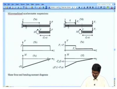
In fact, we can draw this bending moment diagram for this and also shear force diagram. So which is shown in this picture over here the left side picture as I take sections at different points I will see that this vertical shear force V remains constant that turns out to be just V all through from X = 0 to L whereas bending moment it will be 0 here this L–X. This is 0 there and then as we go it is going to be –F or L.
