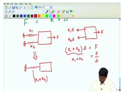
The new spring delta which is F over delta =K1+K2. In other words, this thing I can show it as a single spring which has a stiffness K1+K2. So springs in parallel we will have their stiffness added in order to get the equivalent spring constant.
