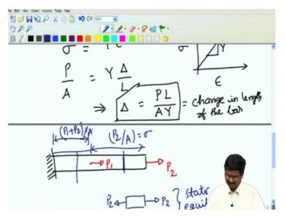
So here if I go back for this portion the stress is going to be P2/area of cross section this is the stress whereas for this portion the stress is going to be P1+P2/area of cross section. So because of this we have to keep in mind that whenever there is an elastic body when there are different forces acting at different points our stress is going to be different because the internal force might be different.
