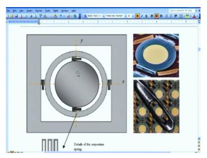
Let us consider one more example before we begin to study this. So here you see an eye of the needle and within that we have lot of these micro mirrors. One of them is shown in a closer view. This particular mirror is schematically shown on the left side and here we have the serpentine beams as shown here each one of those 1, 2, 3, 4. Four of these have this serpentine beams.
