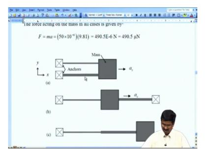
Let us take a mass as shown here connected with 2 bars. So we can get stiffness of this bar and this bar as shown here if I say. The first one we have a stiffness indicated as K which is given by area of cross section Y times L. How did we get this?
