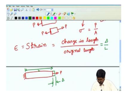
But what we can see is what we can call strain. Strain is defined as the change in length/original length and we use this symbol epsilon to indicate strain. So epsilon is a strain. It is defined as change in length/original length. If we go back to our bar let us draw it again we are fixing the bar at one end and applying a force P because of this force the bar is going to expand a little bit.
