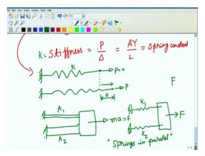
So just as we have done for the previous one now we will have a small bar and a large cross section bar and each of these are connected to a big mass. So this is fixed here this is fixed here area of cross section A1 area of cross section A2 we have the mass on which there is a force the M times acceleration. So this can be represented as 2 springs and there is a mass here. So if I fix the spring I can have spring constant K1 for that K2 for this.
