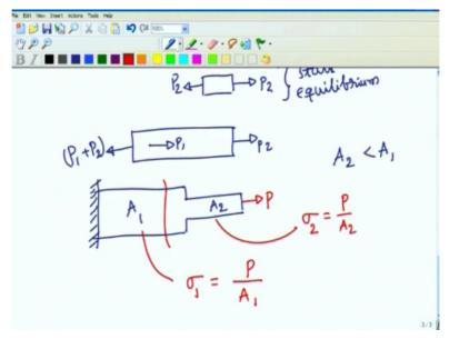
We can also have a situation where I can have a bar with change in area of cross section. So we have here a bar which it is fix at this end area of cross section here is A1, area of cross section here is A2 these are smaller cross section A2 is <A1 if we have that. In this portion anywhere let say we have a force P acting on it. In this portion the stress sigma normal stress sigma is going to be P/A2.
