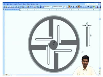
Another example if I take a suspension which is a different kind here we have a central platform, circular in shape here and we have a outer platform and we have beam like structure connected to the central platform to the outside one. In this particular case I can use it to raise the central platform up and down relative to these outer platform so that I can have it like a X, Y or Z stage I can move it in the X direction, Y direction as well as up and down.
