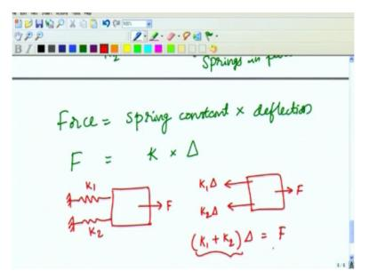
So let us write that so we have the force is = spring constant times deflection of the spring. This is the force F spring constant K times the deflection delta. So now when we have 2 springs like this there will be force acting this way which is K1 times delta if we denote the movement of this mass as delta there will be K1 delta and K2 delta which we will do it here now again.
