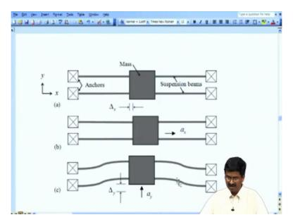
So we have a different kind of suspension we have a mass here and a beams. When there is acceleration in the X direction these beams will only experience axial stresses like bars we just did, but when there is a force or acceleration in the vertical direction then these will deform as shown here. In order to look at those things, we need to again take the beam and show the forces. Now the forces are going to be perpendicular to the beam. So if I take a beam.
