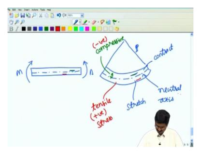
So we have taken a straight beam and we have rotated by applying moment bending moment for this by applying bending moment to rotate it into a circular arch where there is center of curvature and rho which is the radius of curvature. We are saying that there is going to be an axis which will neither stretch nor contract which will call neutral axis. If we have a neutral axis any fiber if you will if you take that and look at it before the ones above have to contract.
