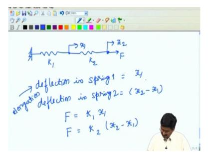
So if I have 2 springs as shown in that picture. Let us call this K1 and another spring this is K2 and if I have a force applied over here this will deflect let us say an amount by displacement X2 this is X1 the deflection in spring 1 this is the deflection or elongation in spring 1 = X because that is what this point is going to move and the deflection in spring 2 is going to be X2-X1. Okay.
