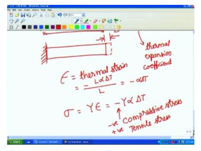
Thermal stress will be what we have written earlier Young's Modulus times the strain which in this case is going to be –Y alpha delta T that will be the thermal stress. Whenever the stress has a negative sign we call it compressive stress. If it is positive, we call it this is negative if it were to be positive we call it tensile stress. So we have compressive stress here and tensile stress. So a bar can also have loading not just thermal loading, but also we can have the mechanical load.
