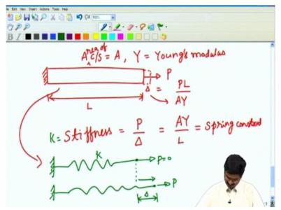
Let us define what stiffness of the bar is. So if I have a bar and I fix here what do you mean by stiffness if I apply a force P let us say the length here is L and the area of cross section is A this is area of cross section A. If it is made of a material whose Young's Modules is Y. We just derived above that the expansion of this bar which we can call delta that was given by P times L/AY that is what we derive a bar.
