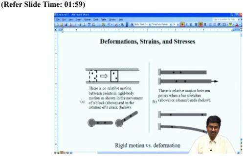
So if you look at this body here which is shown in dash lines and it has been moved to another location where it is shown in solid lines. If I look at these two points before it moved and after it moved the distance between these two points will remain the same if the movement of the body is called a rigid motion. Likewise, if I have a rotating body as shown in the diagram over here.
