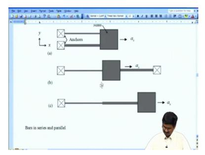
If we take a different scenario we put a narrow bar over here and a wide bar over there even then the 2 springs have the same force acting on the because the same force will act through this bar, same force will act through this bar again these are in parallel. Whereas if I were to attach the springs into end I have shown here the narrow spring and wide spring. I am calling it a spring even if it is a bar.
