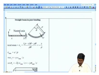
For this let us consider a small straight segment which is under what is called pure bending that is there is a bar and we are applying moment that tries to bend this straight bar into a shape that is shown here. If that bend bar has a radius of curvature rho because it will bend into a circular arch shape the straight one and become circular arch shape that has a radius of curvature rho and an angle theta the sector that is shown here.
