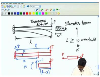
Let say that I show a beam what should be what we call a slender beam. In the case of bars as well as beams we want it to be very long compared to its area of cross section or the dimensions that define the area of cross section. In the case of beam if you want to apply the theory that we are going to develop we want the length of the beam L and let say we take a certain cross section.
