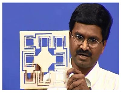
Such a platform I have it here which I will show if you see here in this particular device we have a suspension if I move it in this vertical direction like this you can see it moving and you can also see some other beams observe here for example these beams are deforming. They are not just rigid body movement their motion is not just rigid body motion, but actually deforming as you can see.
