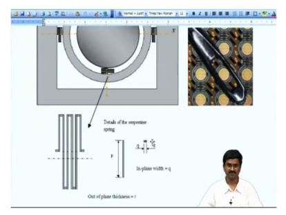
So if we look at the details of this beam suspension it is going to look like this. We have here if I look at this spring it is starting one end corresponds to this end here. Another end corresponds to this and here is our axis. And it can twist about this axis here to make this one rotate about that axis. How do you get an equivalent spring constant or something like this? So looking at these 4 examples let us look at the lumped modeling of these beams.
