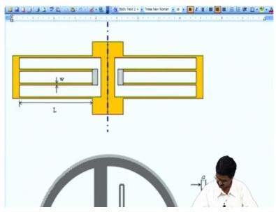
What we have on the screen that we are going to see a suspension. A suspension is called a suspension because the middle I shaped alloy beam that you see here is suspended by a bunch of beams 4 on the left slide, 4 on the right side. These beams suspend this mass so that it can move only in the vertical direction like this where the axis is shown here, but it will have very high stiffness to move in the perpendicular direction in this plane.
