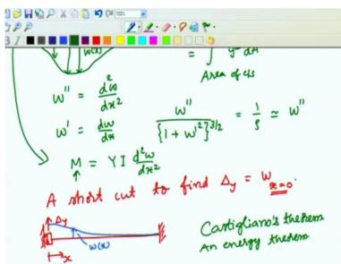
So a shortcut we want to find the shortcut to find delta Y which for us W at X=0 because we have a beam which is fixed at one end and guided at this other end. You want to determine this delta Y. So if my X is starting here at this point X=0 and what we are saying is when this deforms. Let us chose a different color it is going to go to that point we would like to know this is our W.
