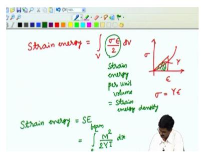
Let us write what this stain energy is? The strain energy is integral of sigma that we introduced earlier stress times strain half of it over the volume of the body. In other words, stress times strain if I were to take a graph where I have stress here strain here if I have a curve like this or a straight line in the case of linear things the slope of this is given by the Young's Modulus because we know that stress=Y times epsilon where Y is the Young's Modulus.
