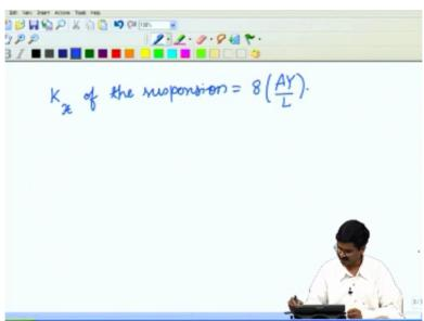
So we can write the total stiffness of this in the X direction of the suspension. This is KX of the suspension as 8 times the spring constant we just derive which was A\*Y/L that gives the Kx. Going back to our figure we have this suspension and this spring constant the X direction which is this Kx we have derived expression. Now if there is a force in the Y direction on it which is again let say MAy
