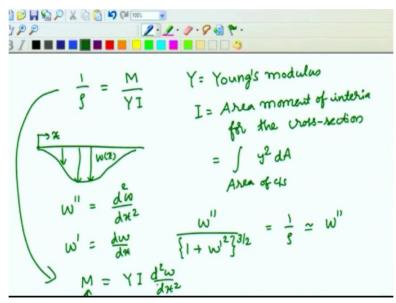
And we also know that I over rho that constant proportionate is here is M/EI. Based on this well let us use YI where Y again is Young's Modulus and I is area moment of inertia for the cross section. So the cross section plays an important role in how much the beam is going to bend because of the bending moment. So we need to have that come here as I which is given by integrating over the area of cross section a quantity Y square DA that is the area moment of inertia.
