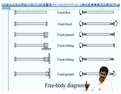
Now let us look at the beams of different boundary conditions. Left side we have shown all of them as fixed. Right side this is completely free so this will not have any reactions at this end at the right end because it is completely free that is called fixed free no reaction moments. So you need to get only these three and for a planar case you have 3 equilibrium X direction can be balance Y direction can be balanced and a rotation can be balanced.
