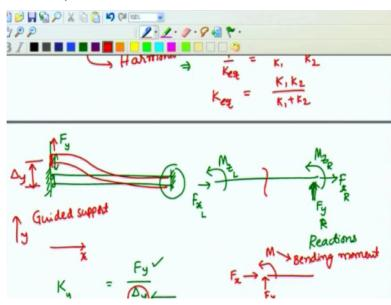
But if I take a section of this anywhere I can again show the vertical reaction and horizontal internal force (()) (36:55) because it is internal and there will be a moment. Notice that all of these we are writing in the positive direction. These are positive X direction, positive Y direction and positive direction for moment either reaction moment or bending moment is counter clockwise.
