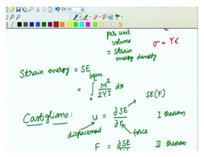
Then what Castigliano's theorem says that the deflection at a point. Let us say U at somewhere is=the derivative of the strain energy with respect to the force correspond to this one. So this is the displacement that we want at a point. At that point if there is a force then we write the strain energy. This strain energy we should write in terms of that force. In fact that will be true for this beam.
