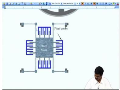
Let us look at one more example. Here the central mass which is called the proof mass we wanted to move in the X direction that is this direction as well as Y direction. So here we have a little coordinate system shown there this is the X direction, Y direction with complete decoupling meaning that when there is a force acting in the X direction Y direction is not affected.
