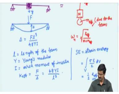
That is, when do we say the stiffness is K for a system if half K times displacement square is = the strain energy stored in that complex elastic system. Then that is the lumped stiffness which we can call K effective. Okay, just recalling what we had discussed in the last lecture. If the strain energy stored in an elastic system if that can be expressed as half K effective times displacement square, then that is the K effective.
