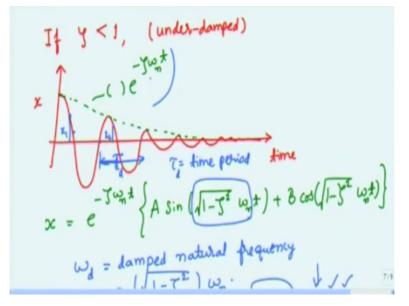
So, we had defined this damping ratio and we actually saw the importance of this damping ratio. This is the second order system if I pert up that a little bit like in a free vibration then it will start at some value and amplitude as it oscillates is going to reduce and that is where this damping ratio applies. There is omega n which is the natural frequency which is dependent on only K effective on inertia effective, m effective.
