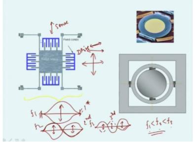
There also more kinds that quick in have one element which is what we kept showing in many lectures that it is a gyroscope. This gyroscope has matched frequencies and it is important to have the match because otherwise at resonance we put it a resonance to have maximum amplitude with minimum effort and the other one also should have the same frequencies.
