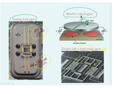
So, how does it look like in reality for a micro machine gyroscopes such as a small chip that I showed a few minutes ago. That might have an element such as what is shown here in 3 different ways, okay. Let us first look at this wheel gyro as it is called, okay this is the wheel gyro. This is Bosch company makes a micro machine wheel gyro and in fact that is what we may be familiar with as a gimbal wheel.
