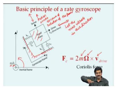
The basic principle of angular rate gyroscope simply lies in the fact that there is a proof mass such as this and that is set to be free to move in 2 directions. We can call this x axis that is in this direction and another is the y axis local and we have intentionally shown that the thing is rotated. If I think of this frame, okay this frame if we think of a box or there a thing that is actually rotating. That is what we shown here.
