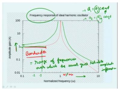
So, the same ratio that kx/F0 if I plot it on the log scale as shown over here. We see that, okay so, let us okay that is log scale and so is this. This is the frequency omega divided by omega n natural frequency it is one that is where the resonance occurs and you see when you log-log plot. If you do that there is a portion which is constant and then it goes like this.
