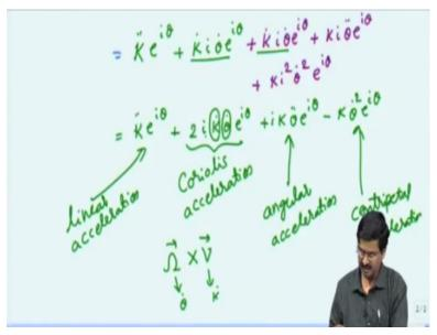
This is linear acceleration. Remember that rod is sliding, the block is siding along the rod and that is linear acceleration and this portion which you can recognize as our centripetal acceleration. Notice that these 2, the first and the fourth term do not have i in them. It is just e power i theta is the direction they just going along the rod but in these other two terms have i in them. They will be perpendicular.
