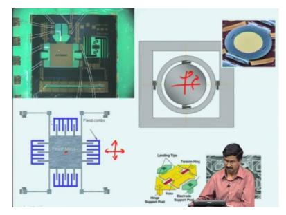
And first we had discussed the motivation for studying vibrations in the context of micro systems. So, this is an accelerometer, a chip and this is a gyroscope that we will talk about today. And here is a mirror that tilts about 2 axis that is as shown here rotation about this axis that is the Y axis if we call vertical axis and horizontal axis and there is a mirror about a single axis this can tilt. So, that is another one.
