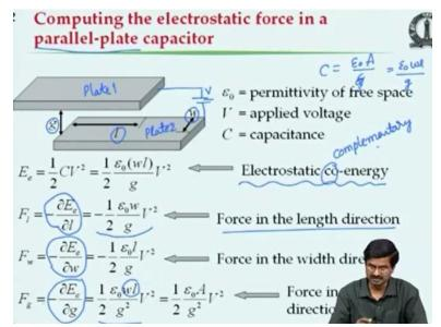
Let us consider a very simple problem of 2 plates that are parallel to each other, which we call parallel plate capacitor. Parallel plate capacitor that means there are 2 plates that are parallel to each other. This is Plate 1 and this is plate 2, based on what we have seen in micro systems until now, you can relate to this type of parallel plate capacitor arrangement in many devices.
