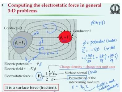
How do we get this formula? What is the basis for it? For that we need to review the basics of electrostatics itself, a very quick review. First, whenever we have conductors as it is shown generally in this, so here we have conductor 1 and there is conductor 2 here. Both of them are at different potentials, the first one is at potential V1 and the second one is at potential V2 and as you know, let us say V1 > V2 then the field lines going from here to there.
