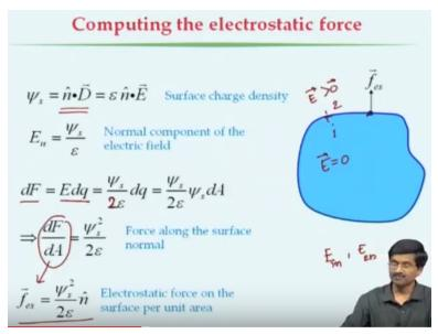
This electric displacement if I take the normal component of that, because electric displacement is going to act everywhere in the domain because electric field everywhere when you come to the boundary of the conductor that electric displacement if I take the normal of this D, dot product with the, if I take normal component of D, which is simply the dot product of D and the normal vector what we get is nothing.
