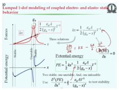
So, you have to analyse that we need to discuss the stability of the equilibrium solutions and to see the stability, let us look at the forces. The mechanical force, which is shown as a straight line here and the other curved one is the electro static force. You can see that when x = g 0, it is going
