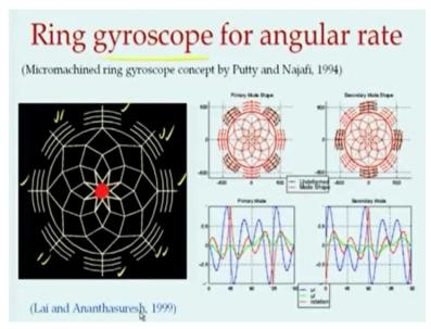
So this is a different kind of a ring gyroscope. Here, we have the same central post as it is shown. Here, it is fixed only there, in the rest of the structure is free to move. Here we see that, to the ring there are lot of these cones attached to it and there are 2 degenerate mode shapes for it. One shape is such that this one, this one, this one and this one. That is these 4 sets of cones oscillate that is as shown over here.
