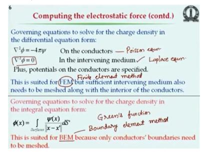
Now we already said that for the intervening medium, we need to solve this equation, which we call Laplace equation and inside the conductors there usually no charge, if they are worked to be charged or on the conductor there want to be some charge we have to use this one, Del Square Phi = some non-0 value, which we call Poisson equation. So that we can compute the potentials and then from the (()) (22:27) electric field from that, the vector D and then the surface charge and then the force.
