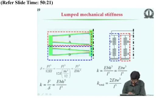
For that, we need to first estimate, let us say before we go to derivational modeling, we have to just estimate the pull in voltage, for that we try, we treat this suspension as 4 beams on this side, which are fixed and guided, fixed and guided, a lump modern technique that we have discussed
