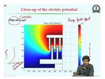
So on to compute, the pull in voltage for the 3 dimensional structure, such as this, we have to start with some initial V value, voltage we have to start some value and then raise it to another value, raise to another value and then see how this placement looks like. If the pull in is going to occur, so what we would find is that this placement initially will increase like that and sudden at some point, it just goes to infinity.
