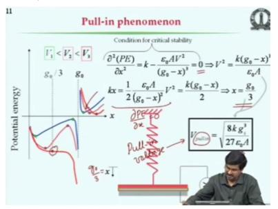
So it is clear that between these 2 problems, that is between that these 2 solutions, which is the first solution, second solution, the plate will choose this one that is closer with x = 0, the plate is moving and it is (()) (34:25) this. And we have already said that third solution is more than g 0, so we do not worry about it. Now let us say I increase this voltage from V 1 to let us say V 2, which is larger than V 1.
