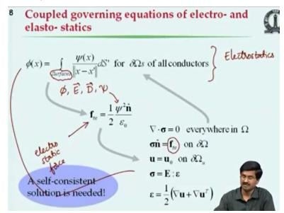
Let us see that in the form of equations. Here we are showing the integral form of the electrostatic equation. This is electrostatics and once we solve it we will get the potential and then we will get the electric field and then will get the electric displacement, we get a surface charge density Psi and that Psi goes here we get the electrostatic force.
